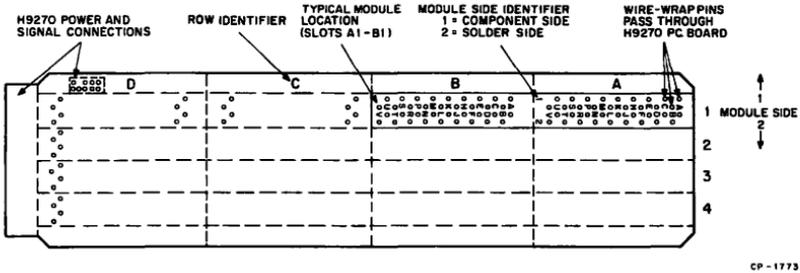
**Figure 3 LSI-11 Backplane Module Pin Identification**
