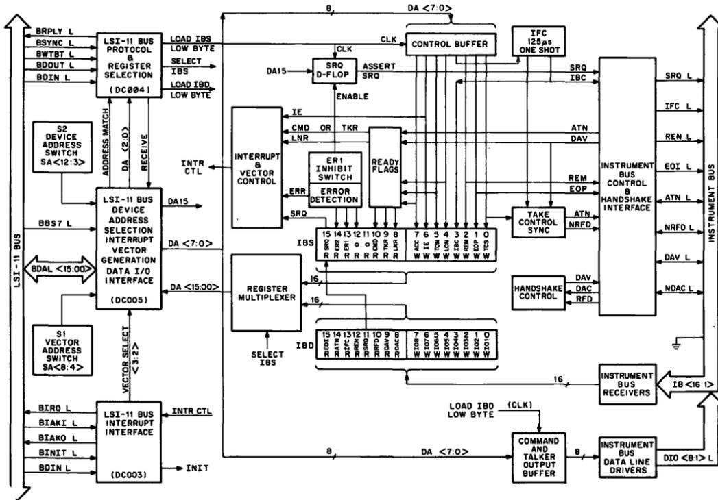
Figure 1 IBV11-A Functional Block Diagram
