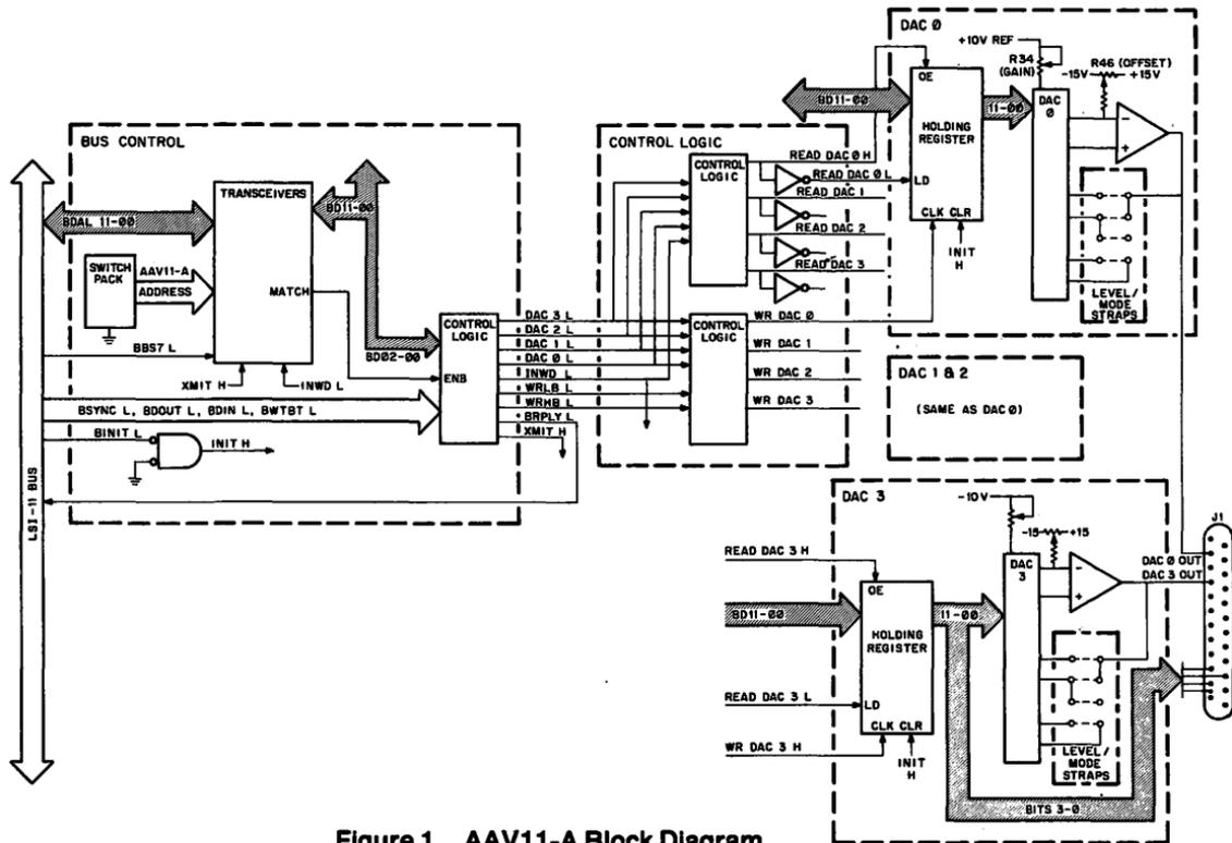
Figure 1 AAV11-A Block Diagram
