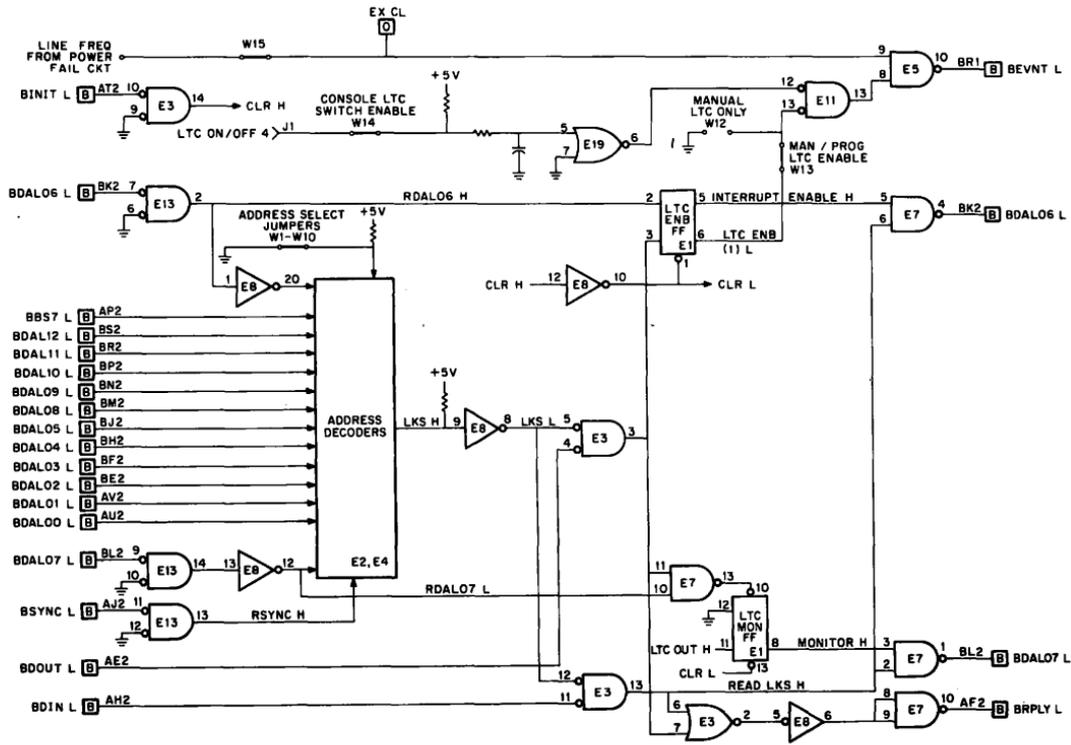
Figure 4 Programmable Line-Time Clock Circuits
