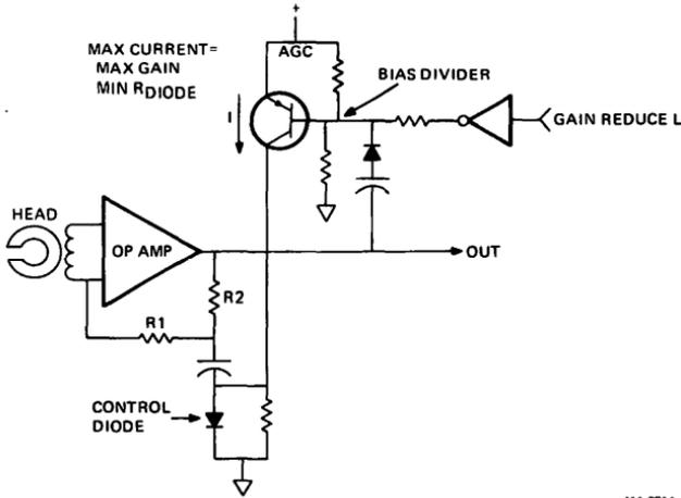
Figure 19 Read Amplifier and Automatic Gain Control
