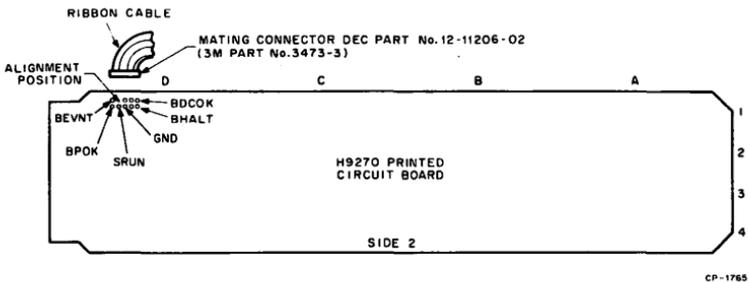
Figure 4 H9270 Backplane Signal Connections (Pin Side View Shown)
