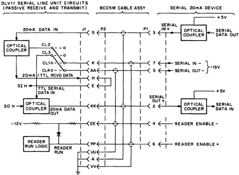
Figure 10 Passive 20 mA Current Loop Interface
