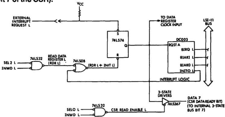
Figure 11 Typical Interrupt Request
