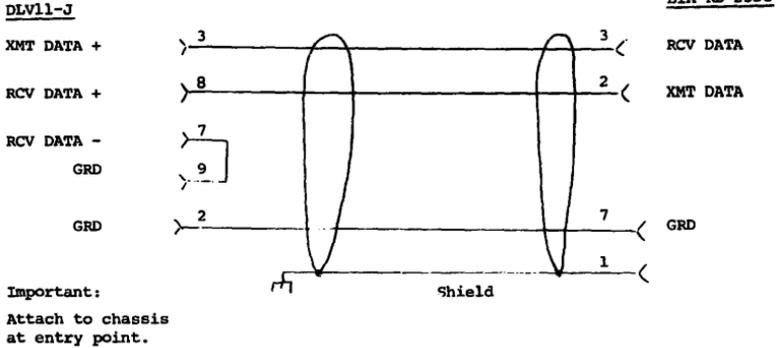
Figure 8 BC20N-05 "Null Modem" Cable
