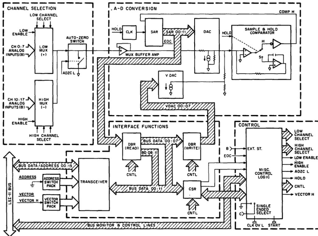
Figure 1 ADV11-A Functional Block Diagram
