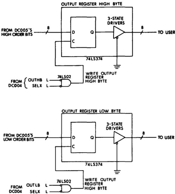
Figure 6 Example of Output Register
