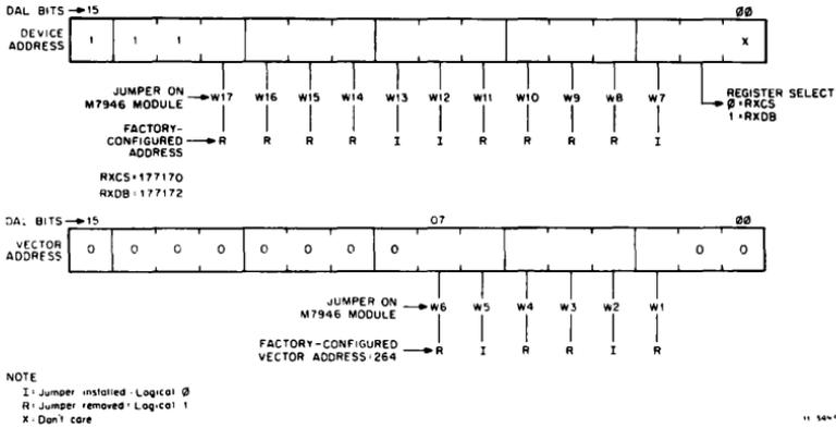
**Figure 2 Device Register Address and Interrupt Vector**
