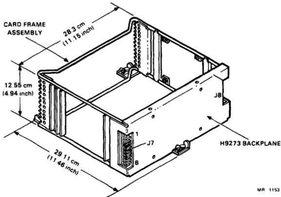
Figure 1 H9273-A Backplane Logic Assembly
