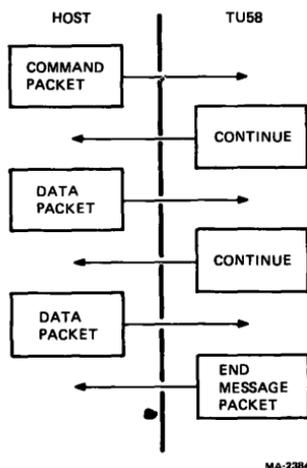
Figure 2 An Exchange in Radial Serial Protocol
