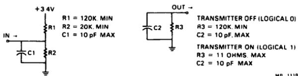
Figure 1 Bus Driver and Receiver Equivalent Circuits
