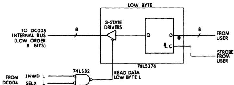
Figure 7. Example of Input Register (BYTE)
