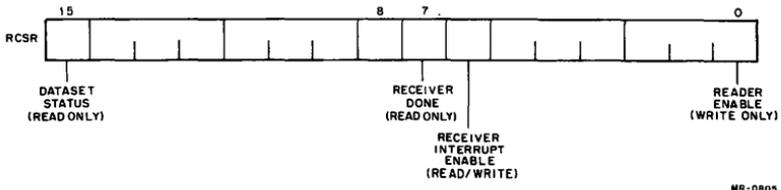
Figure 3 Receiver Control/Status Register (RCSR)
