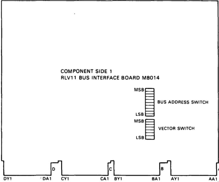
Figure 2 RLV11 Bus Interface Module (M8014)
