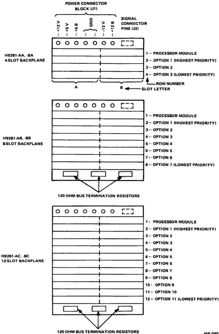
Figure 5 H9281 Option and Connector Locations (Module Side)
