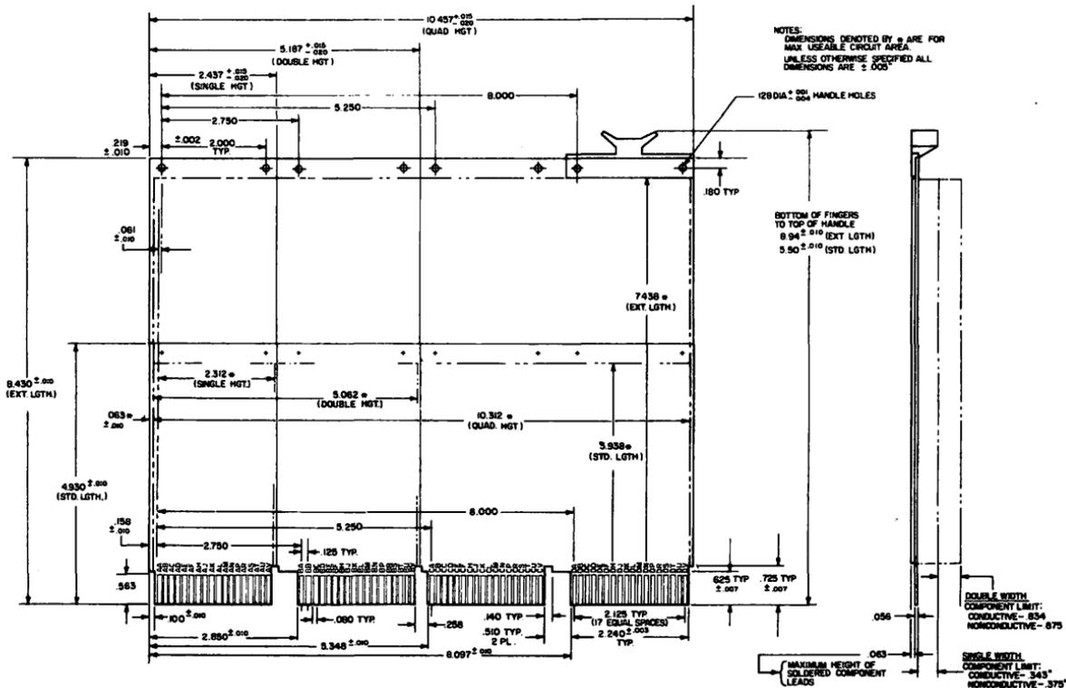
Figure 1 Module Dimensions
