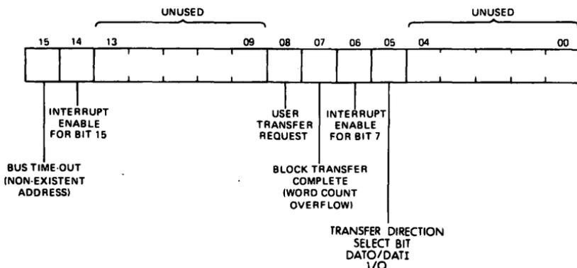
Figure 6 Control/Status Register (CSR) Format
