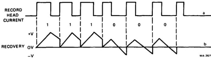
Figure 18 Data Encoding and Decoding
