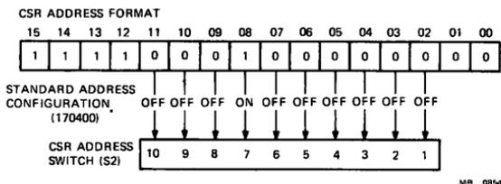
Figure 3 CSR Switch-Selectable Address
