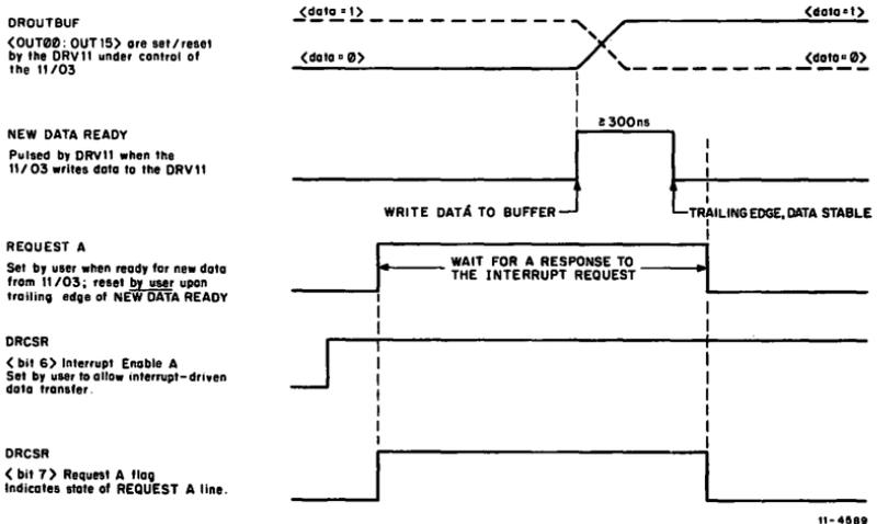
Figure 9 DRV11 Interface Signal Sequence
