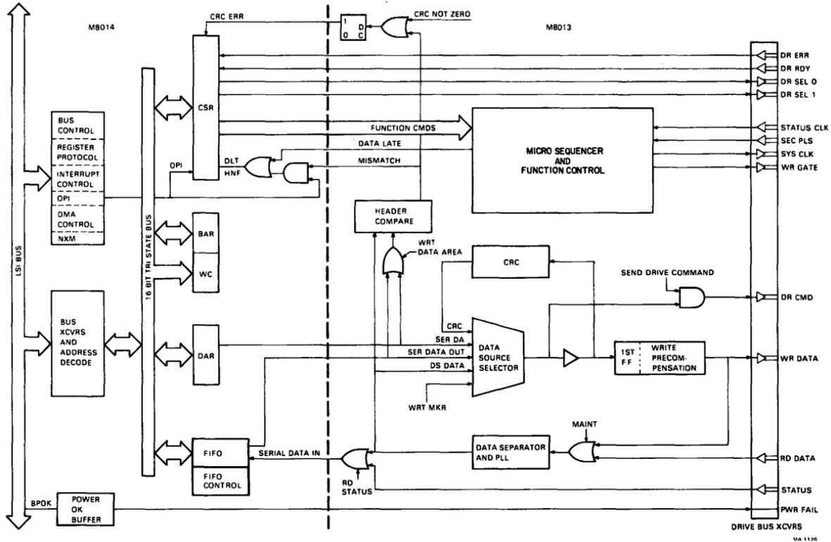
Figure 1 RLV11 Controller Simplified Block Diagram
