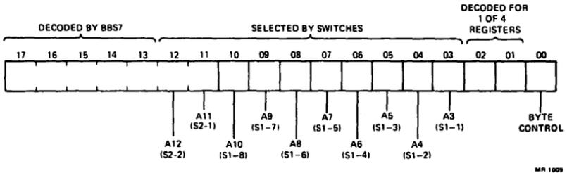
**Figure 2 Device Address Select Format**
