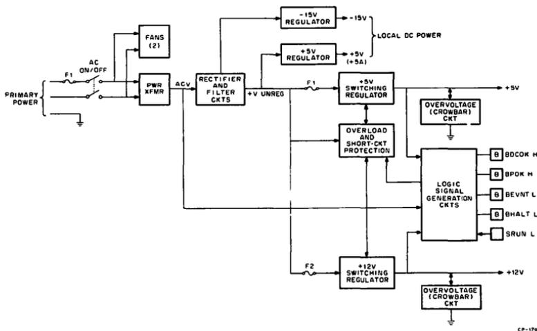
Figure 4 H780 Power Supply Block Diagram
