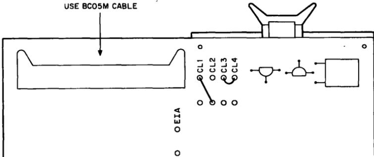
Figure 11 20 mA Passive Current Loop Jumper Configuration
