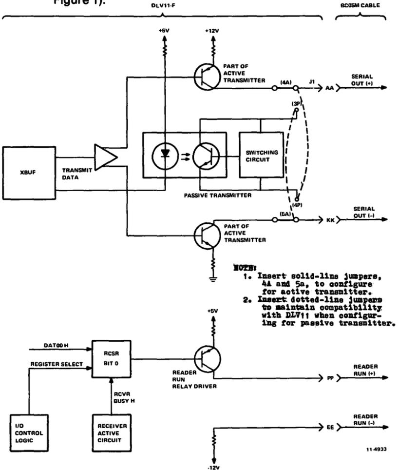
Figure 10 20 mA Transmitter and Reader Run Circuits
