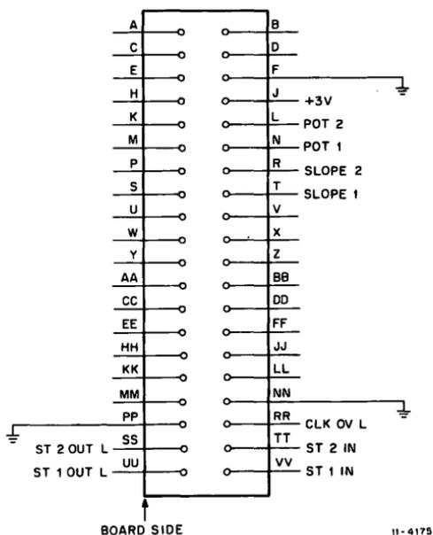
Figure 8 J1 40-Pin Connector Pin Assignments
