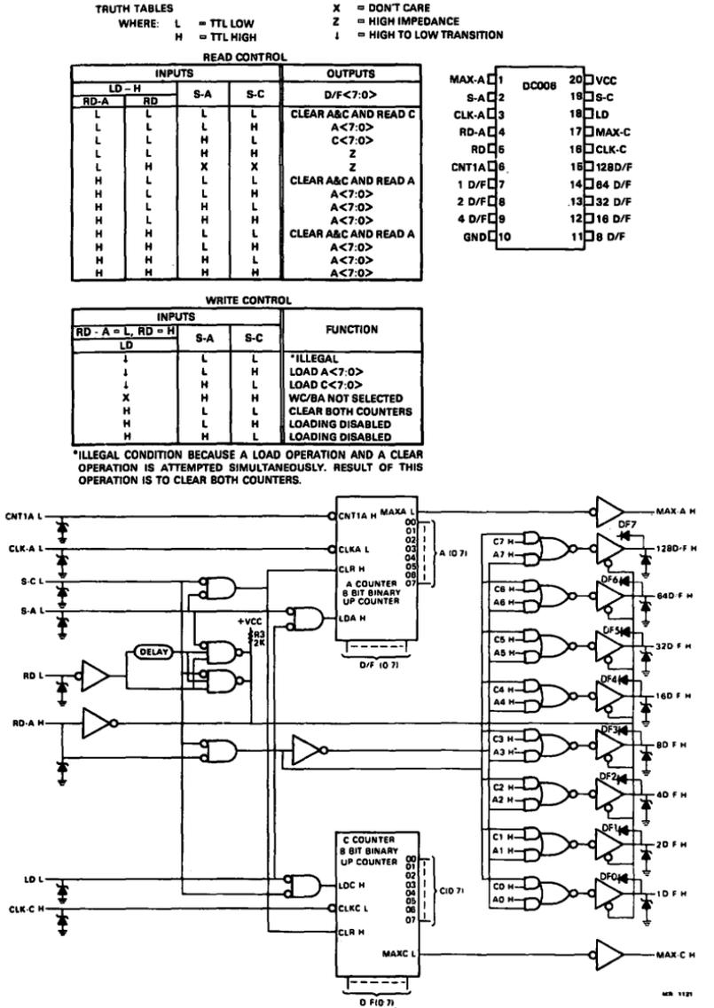
Figure 8 DC006 Simplified Logic Diagram
