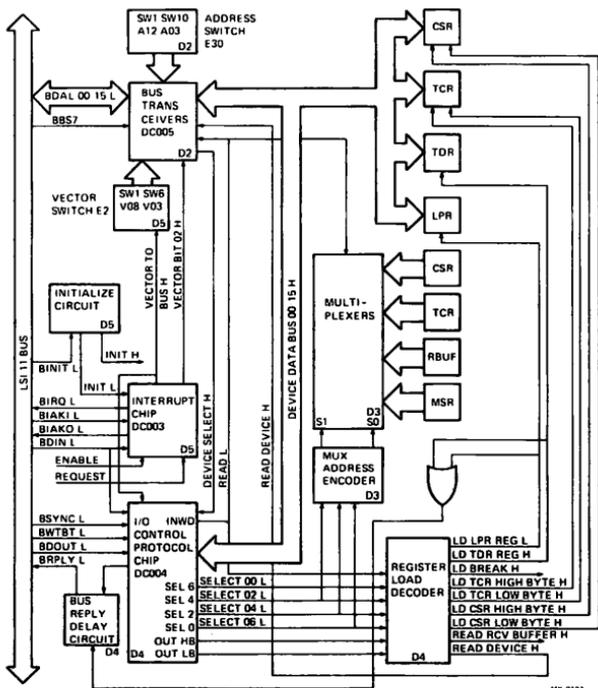
Figure 1 Bus Interface, I/O Control, and Interrupt Logic
