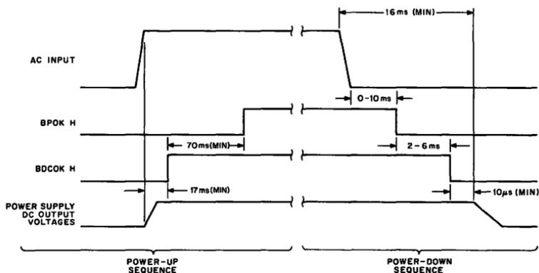
Figure 2 Power Signal Sequence Timing
