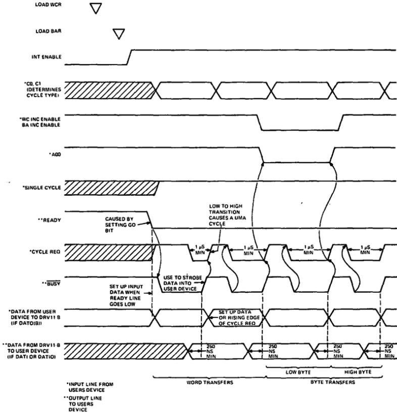
**Figure 5 DRV11-B Timing: Single Cycle, Asynchronous, Program-Initiated**
