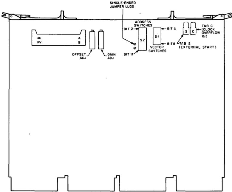
Figure 2 ADV11-A Connectors and Switches
