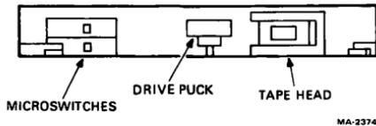
Figure 7 View Into Tape Drive Cartridge Slot
