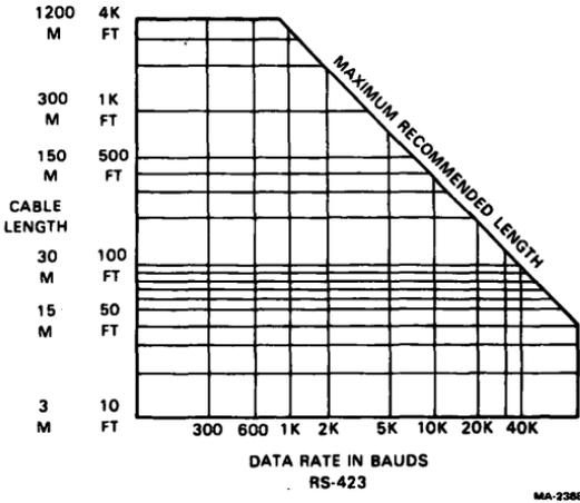
Figure 12 Data Rate and Cable Length for RS-423
