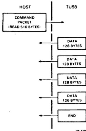
Figure 8 Read Command Packet Exchange
