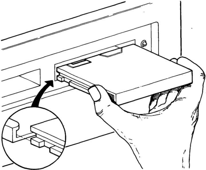
Figure 1 Loading a Cartridge
