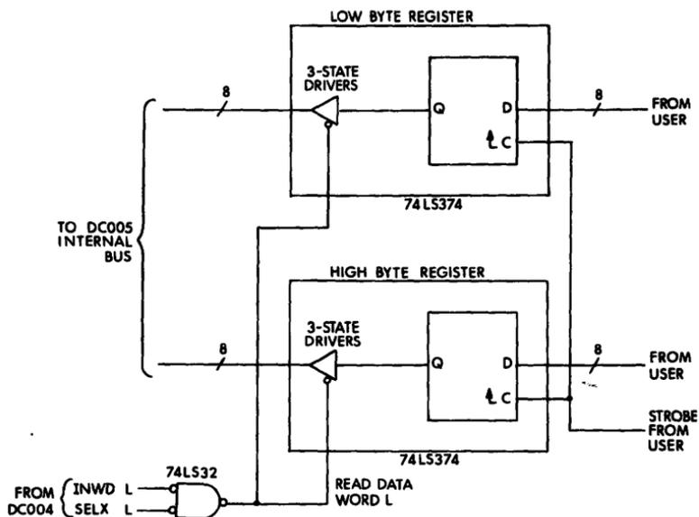
Figure 8 Example of Input Register (WORD)
