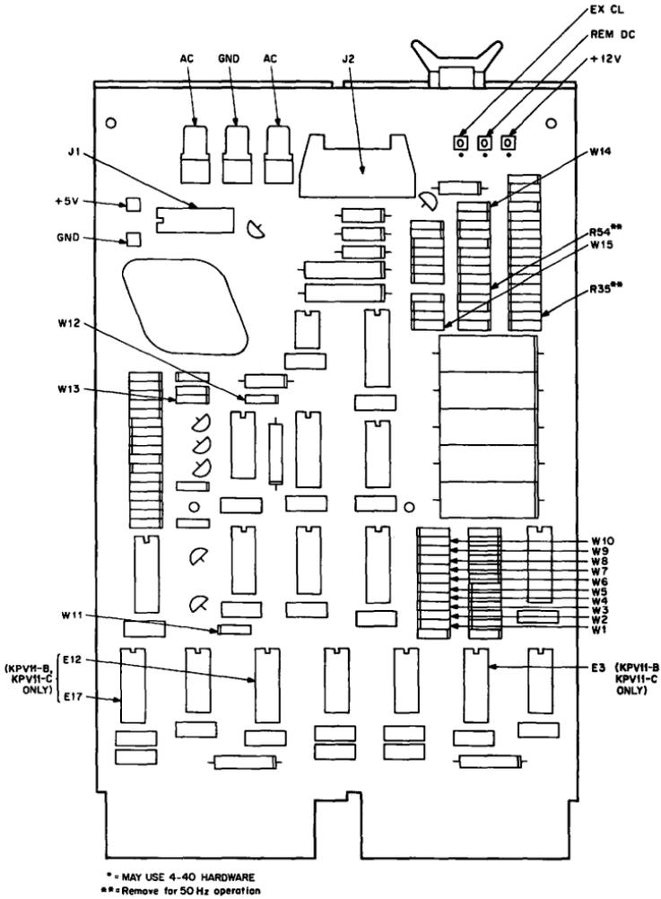
Figure 7 Jumper, Connector, Resistor, and Pad Locations
