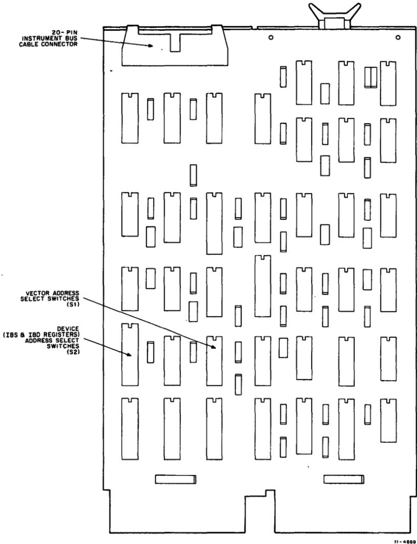
Figure 4 IBV11-A Module Switch Locations
