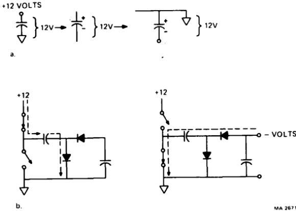
Figure 20 Simplified Charge Pump
