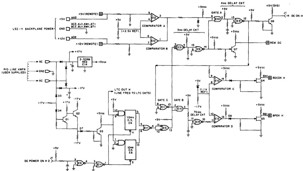
Figure 3 Power Signal Sequence Circuits
