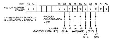
Figure 44-3 • LPV11 Interrupt Vector Selection Jumpers
