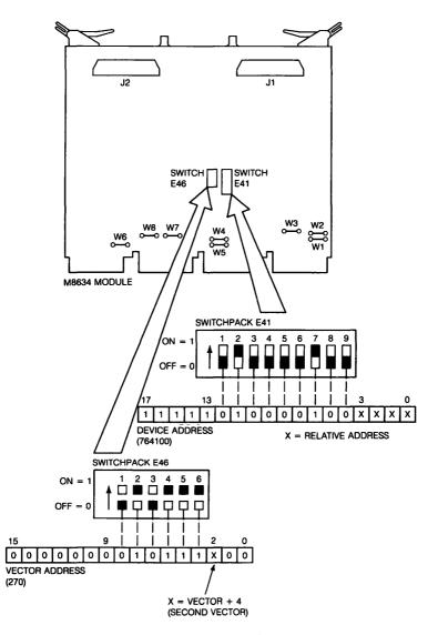
Figure 42-1 • M8634 Module Layout
