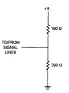
Figure 63-2 • Typical 120-Ohm Bus Termination
