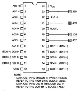
Figure 17-3 • MXV11-A ROM Socket Pin Assignment
