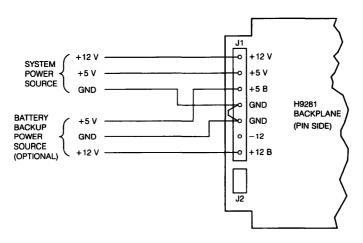
Figure 62-3 • H9281 Power Connections
