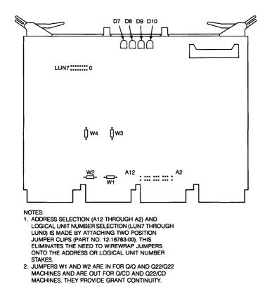
Figure 47-1 • RQDX1 Controller Module Jumper and LED Locations
