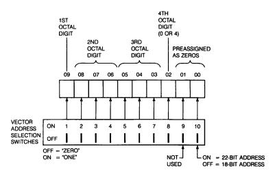
Figure 40-3 • DRV11-WA Interrupt Vector Address Selection
