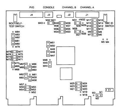
Figure 7-1 • KXT11-CA Jumper Layout
