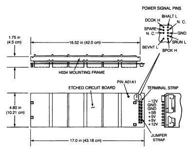
Figure 57-3 DDV11-B Power Wiring
