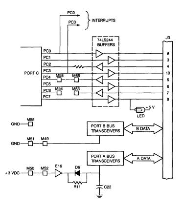
Figure 6-3 • SBC-11/21-PLUS Parallel I/O Configurations
