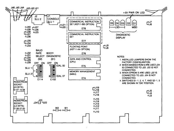
Figure 4-1 • LSI-11/23-PLUS Jumper and Switch Locations
