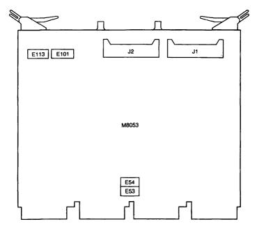
Figure 29-1 DMV11 Switch Locations (M8053 Module)
