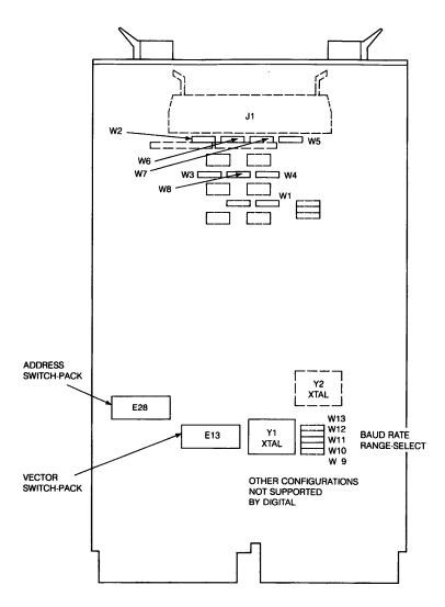
Figure 24-1 • DZQ11 Jumper and Switch Locations
