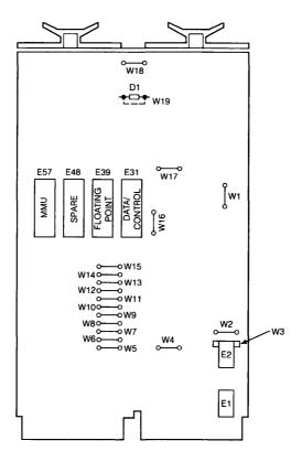
Figure 3-1 • LSI-11/23 Jumper Locations (Rev. A)
