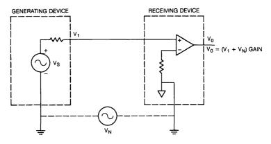
Figure 34-4 • Single-Ended Analog Input
