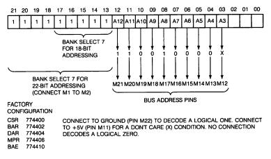
Figure 45-2 RLV12 Device Address Format
