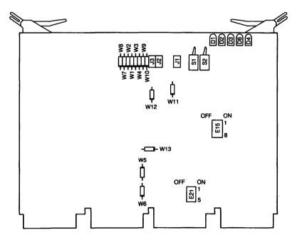
Figure C-1 BDV11 Switch and Jumper Locations
