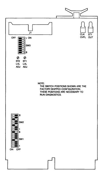
Figure 36-1 • KWV11-C Module Layout
