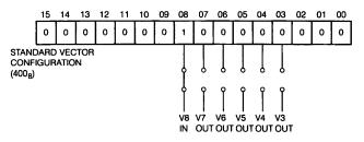
Figure 35-3 • Selecting AXV11-C Interrupt Vector Address
