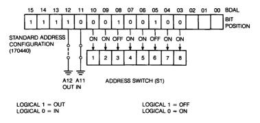
Figure 33-2 Selecting AAV11-C Device Address
