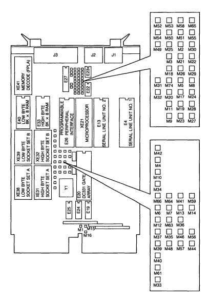
Figure 6-1 = SBC-11/21-PLUS Module Layout
