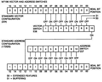
Figure 50-2 • TSV05 Vector and Device Address Selection
