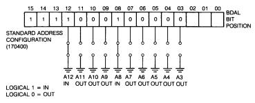
Figure 34-2 • Selecting ADV11-C Device Address
