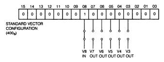
Figure 34-3 - Selecting ADV11-C Interrupt Vector Address
