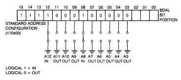
Figure 35-2 • Selecting AXV11-C Device Address
