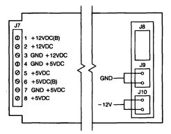
Figure 60-2 • H9273-A Power Connections
