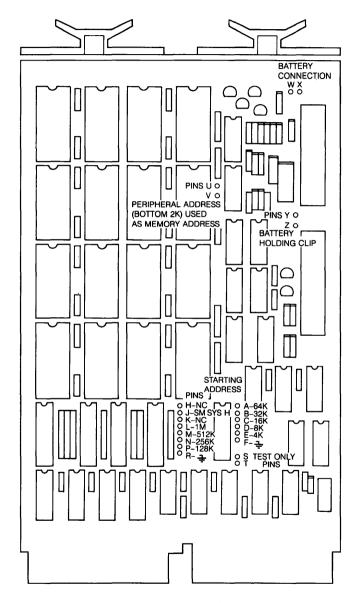
Figure 9-1 • MCV11-D Module Layout
