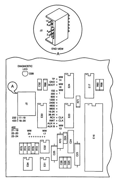
Figure 51-1 • TU58 Controller Board
