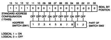
Figure 36-2 Selecting KWV11-C Device Address
