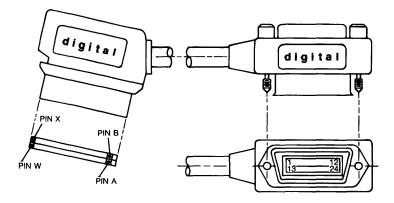
Figure 41-4 • BN11A Instrument Bus Cable
