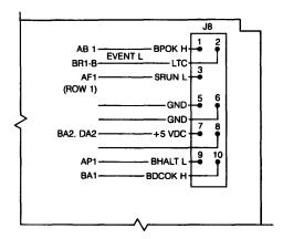
Figure 60-3 • H9273-A Signal Connections
