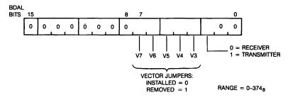
Figure 21-3 = DLV11 Interrupt Vector Address Selection
