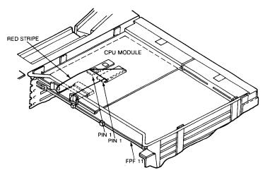
Figure 3-4 • FPF11 Cable Layout in LSI-11/23 System
