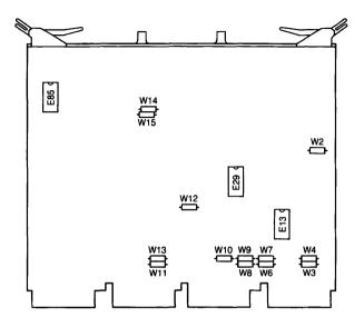
Figure 26-1 • KMV11-A Jumper and Switch Locations
