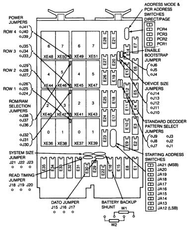
Figure 11-1 • MRV11-D Jumper and Switch Locations
