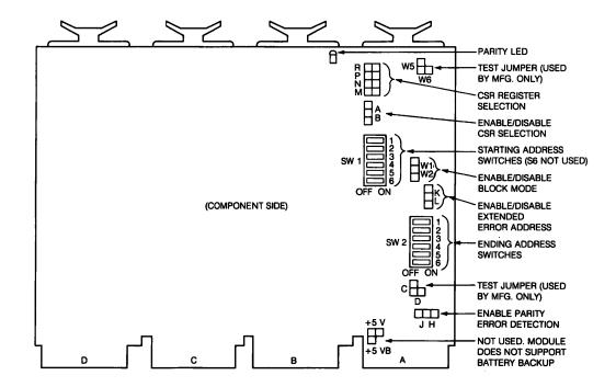
Figure 15-1 • MSV11-QA (Etch Rev A) Switches and Jumpers
