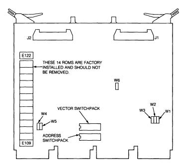
Figure 50-1 • TSV05 Interface Module Switch and Jumper Locations
