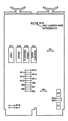
Figure 3-2 = LSI-11/23 Jumper Locations (Rev. C)
