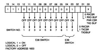
Figure 31-2 Device Address Selection
