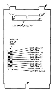
Figure 46-1 • RQC25 Component Layout
