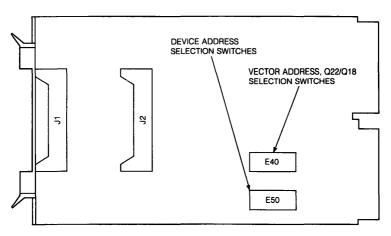
Figure 40-1 • DRV11-WA Connector and Switch Locations
