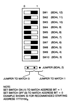
Figure 46-2 • RQC25 Address Switch/Jumper Configuration
