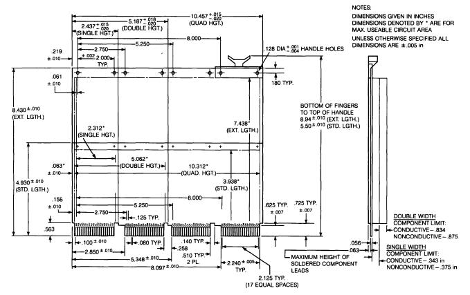
Figure 1-2 • O-bus Module Dimensions
