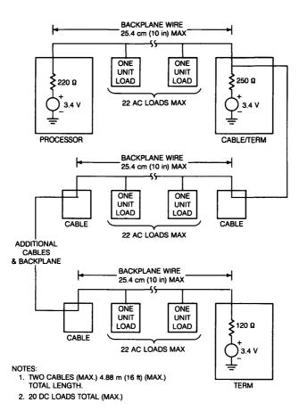
Figure 52-2 • Multiple Backplane Configuration
