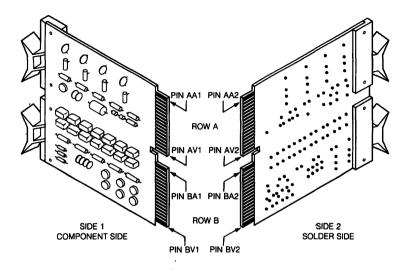
Figure 1-1 • Dual-Height Module Contact Pin Identification
