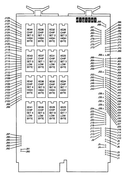
Figure 10-1 = MRV11-C Wirewrap Pin Locations
