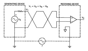
Figure 34-6 • Differential Inputs
