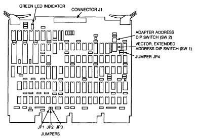
Figure 49-1 • TQK25 Switch and Jumper Locations
