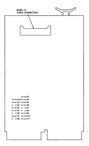
Figure 48-1 • RXV21 Device and Vector Address Jumpers
