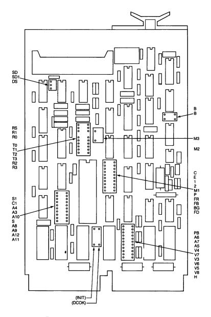
Figure 22-1 DLVE1 Revision D Etch Jumper Locations
