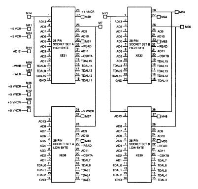
Figure 6-4 SBC-11/21-PLUS Socket Sets A and B Interconnection
