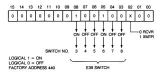
Figure 31-3 • DUV11 Interrupt Vector Selection
