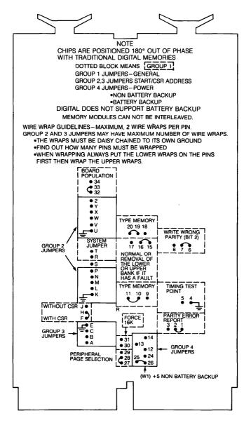
Figure 13-1 • MSV11-L Memory Module Jumpers
