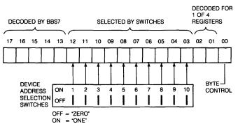
Figure 40-2 • DRV11-WA Device Address Selection
