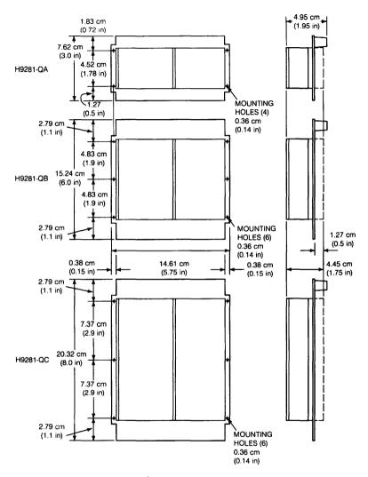
Figure 62-1 • H9281-Q Mounting Dimensions
