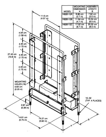
Figure 62-2 - H9281-Q Mounting Dimensions
