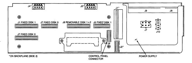
Figure 56-3 • Signal Distribution Printed Circuit Board Layout
