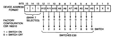
Figure 25-2 DZV11 Device Address Selection
