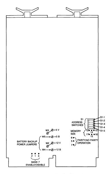
Figure 12-1 • MSV11-D, MSV11-E Switch and Jumper Locations
