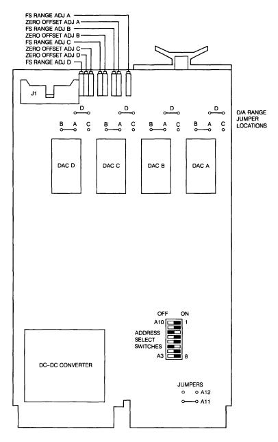
Figure 33-1 • AAV11-C Physical Layout
