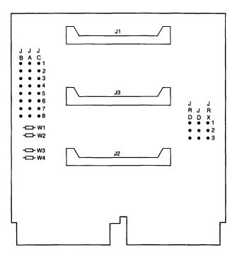
Figure 47-4 • RQDX1-E Extender Module Jumper Locations
