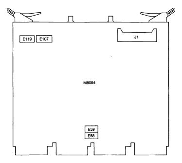
Figure 29-2 • DMV11 Switch Locations (M8064 Module)
