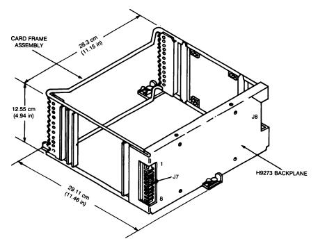
Figure 60-1 • H9273-A Backplane Logic Assembly
