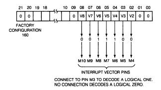
Figure 45-3 • RLV12 Interrupt Vector Format
