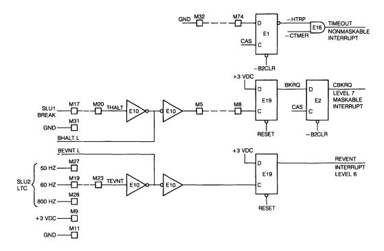
Figure 6-2 • SBC-11/21-PLUS Interrupt Configurations
