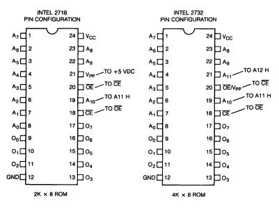
Figure 10-5 • 2K × 8 and 4K × 8 Pin Configurations
