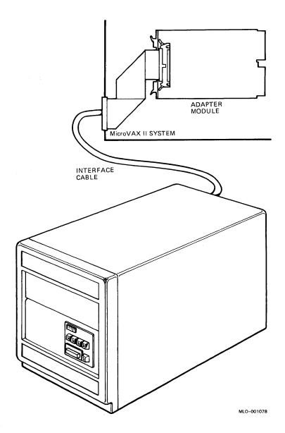
The RC25 uses a KLESI (M7740) adapter module. Use DIP switchpack E58 on the KLESI to set the CSR address (Figure 2). The CSR address factory configuration, and an address for a second KLESI module, follow Figure 2. The interrupt vector is set under program control.
