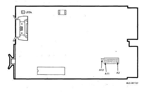
**NOTE:** If a system contains an RQDX2 or RQDX3 controller, this controller must use the first MSCP address (17772150), and the KRP50 must use a floating address.
