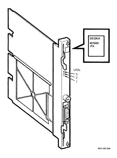
**CAUTION:** Static electricity can damage integrated circuits. Use the wrist strap and antistatic mat found in the Antistatic Kit (29–26246) when you work with the internal parts of a computer system.
