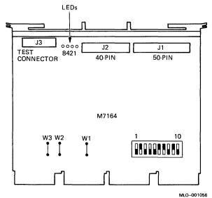
Figure 1: KDA50–Q Processor Module Layout (M7164)
