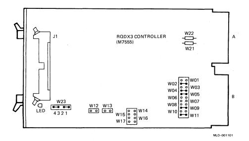
**CAUTION:** Static electricity can damage integrated circuits. Use the wrist strap and antistatic mat found in the Antistatic Kit (29–26246) when you work with the internal parts of a computer system.
