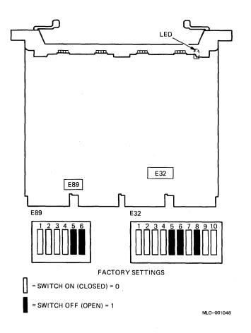
Figure 1: DSV11–S Module Layout (M3108–PA)
