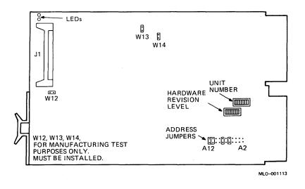
The hardware revision level DIP switch is set to match the module revision level stamped on the back of the module. Make sure the switch setting is correct. The eight switches in this DIP switch represent a binary-weighted value, as listed in the following table:
