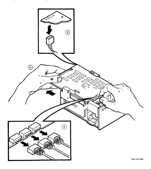
Figure 4: Removing the RD51 Read/Write Board
