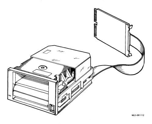
Figure 1: TK50 Tape Drive Subsystem, BA23 and BA123 Enclosures
