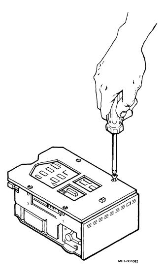
3. Using a 3/32-inch Allen wrench, remove the four screws that hold the read/write board to the RD51 drive (Figure 3).
