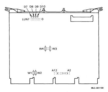
Figure 2 shows jumper and LED locations for the RQDX3.
