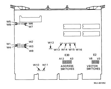
Figure 1: DZV11 Module Layout (M7957)
