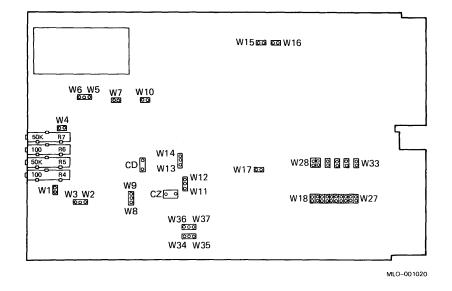
Figure 1: AAV11–D Module Layout (A1009)
