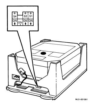
The device electronics board is the only part of an RD53 drive that you can replace. Remove the RD53 device electronics board as follows:
