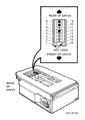
The read/write board is the only part of an RD51 drive that you can replace. Replace the RD51 read/write board as follows:
