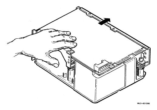
8. Swing the board up as shown in Figure 17. You may have to pull the bracket back slightly; do not pull the bracket back more than is necessary to remove the board. Do not flex the PCBA when removing it.
