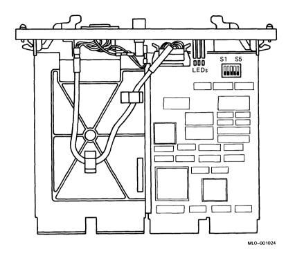
Figure 1: DELQA-S Module Layout (M7516-PA)
