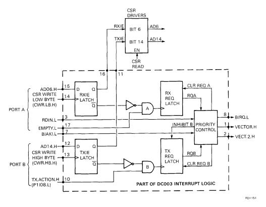
Figure 4-17 Interrupt Logic
