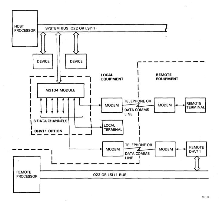
Figure 1-2 Example of DHV11 Configuration
