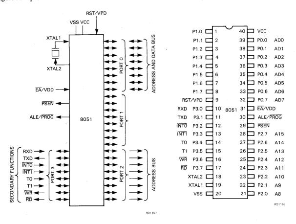
Figure A-2 8051 Symbol and Pinout Diagrams
