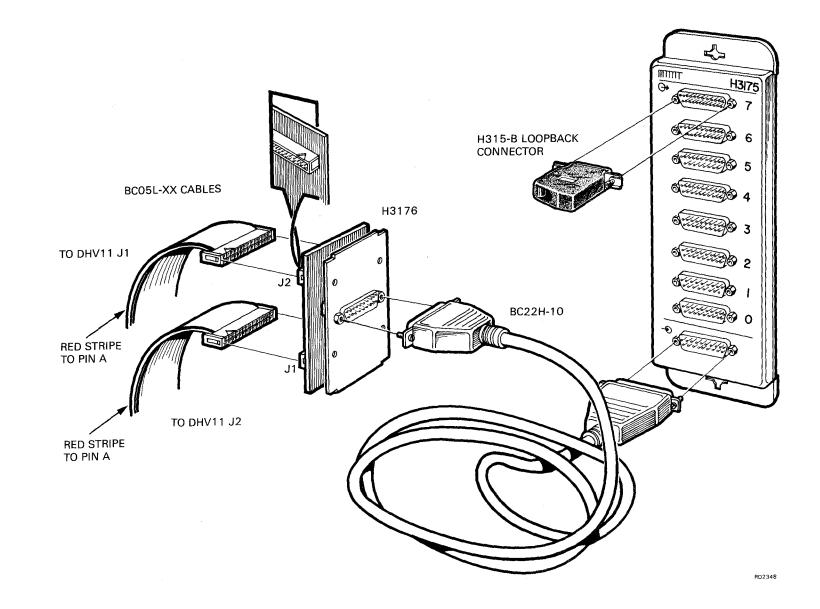
Figure E-2 DHV11 Remote Distribution Panel Cabinet Kit
