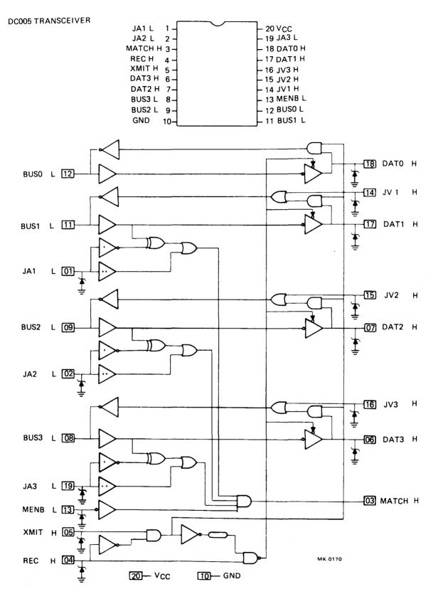
Figure A-13 DC005 Simplified Logic Diagram
