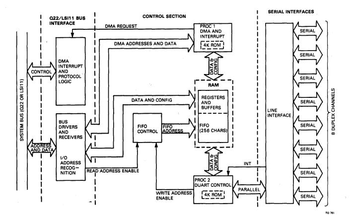
Figure 1-5 DHV11 Functional Block
