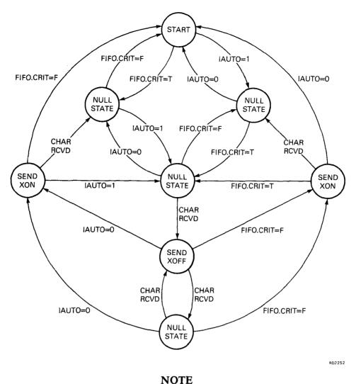
FIFO.CRIT is set true (T) when the FIFO level rises to three-quarters full, and is again set false (F) when the FIFO level falls below half full.
