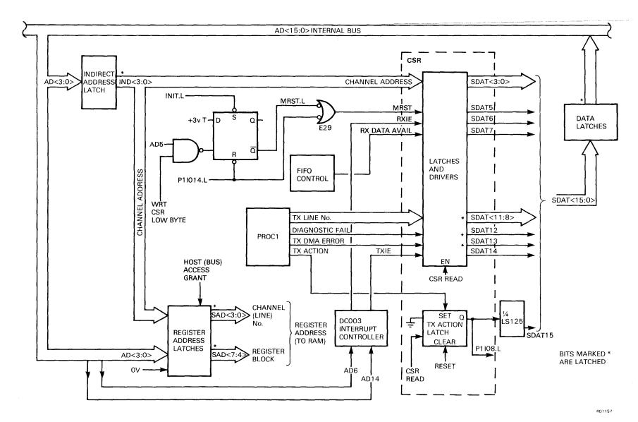
Figure 4-20 CSR and Register Address Circuits
