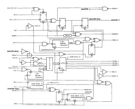
Figure A-15 DC010 Simplified Logic Diagram
