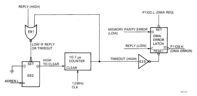
Figure 4-13 DMA/Memory Error Generation
