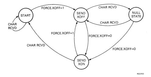
Figure D-3 Program-Initiated Flow Control
