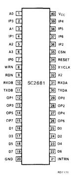
Figure A-7 SC2681 Pin-Out Diagram
