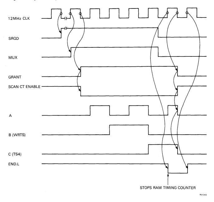
Figure 4-19 Store Access Timing Cycle
