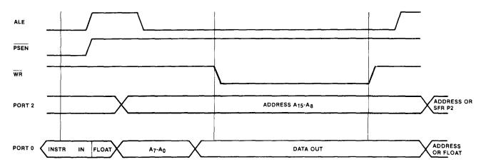
Figure A-5 Data Memory Write Cycle
