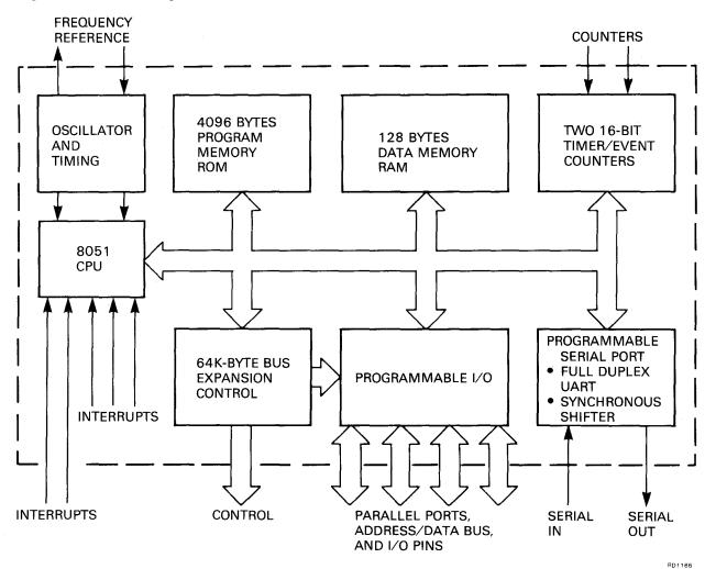
Figure A-1 8051 Block Diagram
