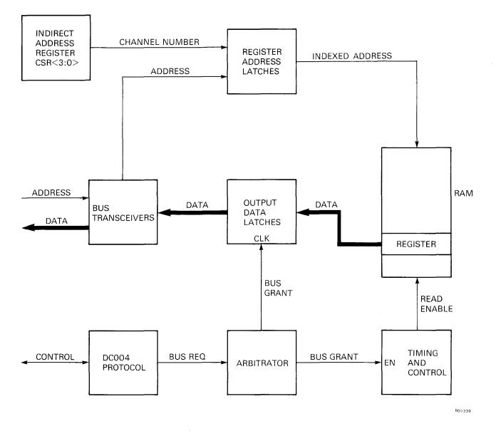
Figure 4-8 Reading from a Register
