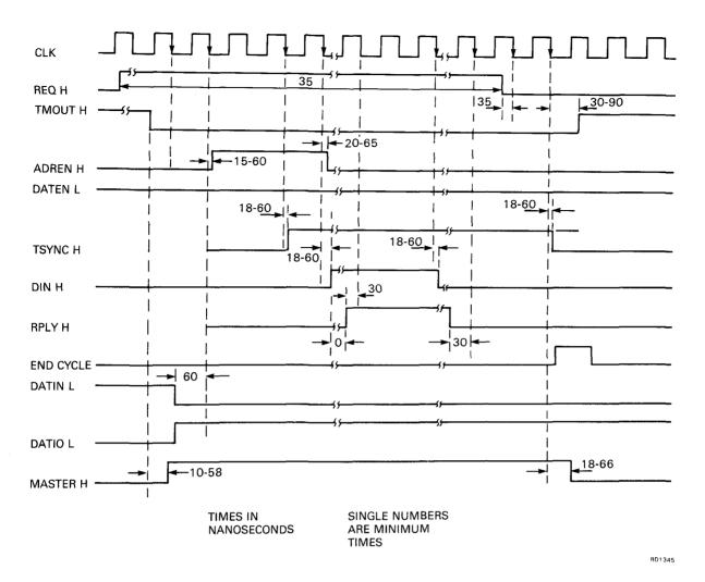
Figure A-19 DC010 Timing Diagram
