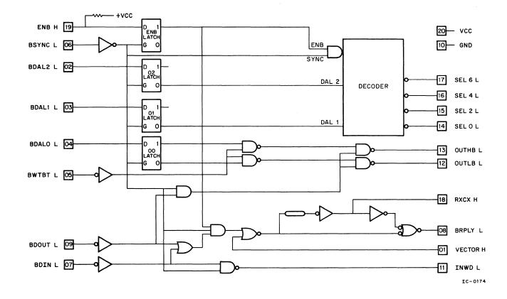
Figure A-4 DC004 Simplified Logic Diagram
