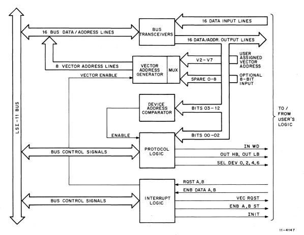
Figure 1 DRV11-P Basic Block Diagram
