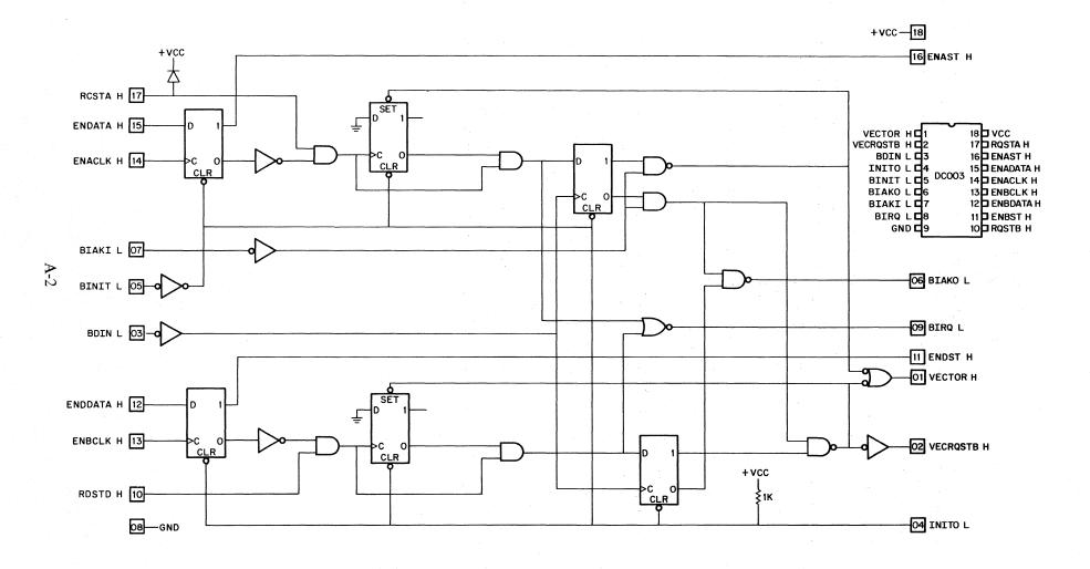
Figure A-1 DC003 Simplified Logic Diagram
