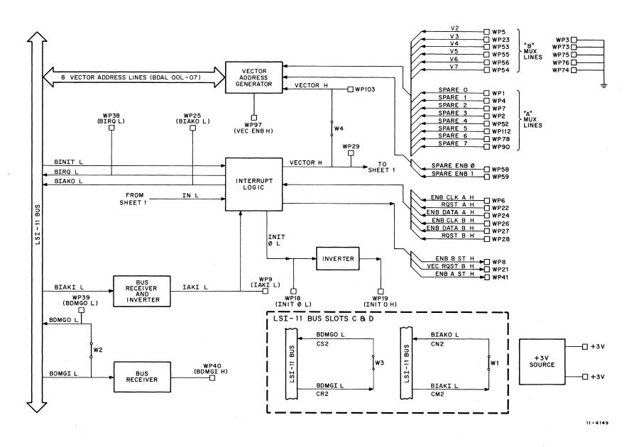
Figure 2 DRV11-P Block Diagram (Vector Address Generator and Interrupt Logic) (Sheet 2 of 2)
