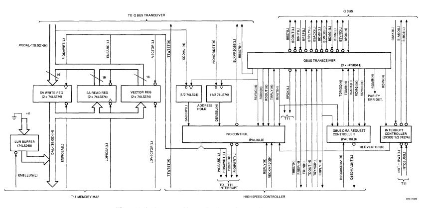
Figure 2-6 Interrupt Vector Register, SA Registers and QBus Interface Logic
