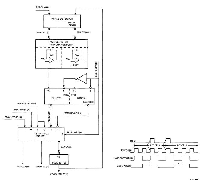
Figure 2-3 Phase Locked Loop Logic
