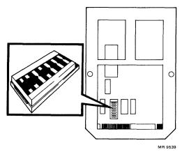
Figure 6-2 RD51 Disk Drive Read/Write Printed Circuit Board
