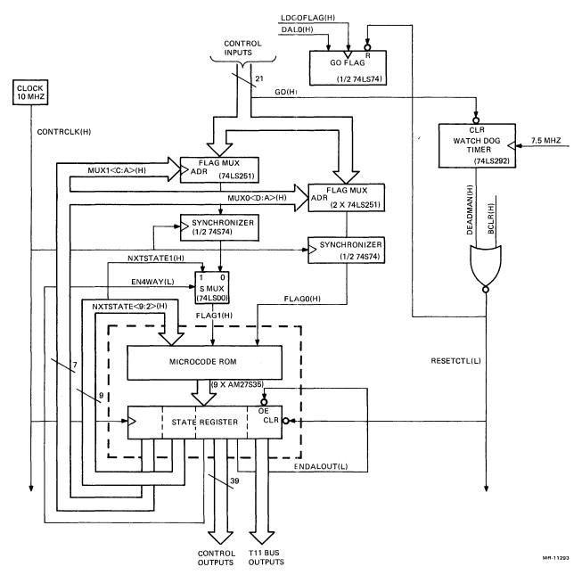
Figure 2-8 Main High-Speed Controller Architecture
