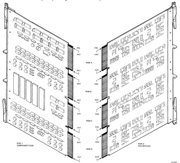
Figure A-1 Quad Module Contact Finger Identification
