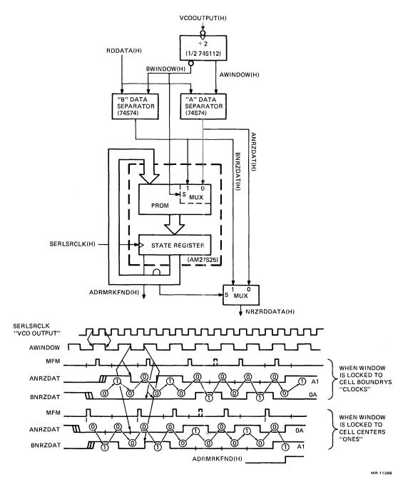
Figure 2-4 Data Recovery and Sync Mark Detector Logic
