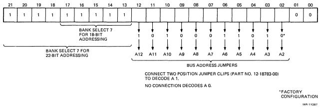
Figure 3-2 RQDX1 Address Selection Jumper Format
