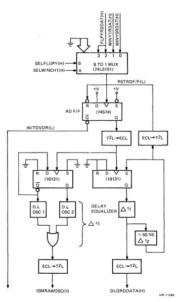
Figure 2-2 Shuffle Step Oscillator
