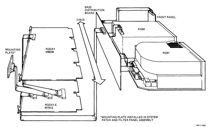
Figure 3-6 RQDX1-E Extender Module Connections
