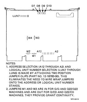
Figure 3-1 RQDX1 Controller Module Jumper and LED Locations
