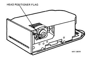
Figure 6-3 RD51 Disk Drive Head Positioner Flag
