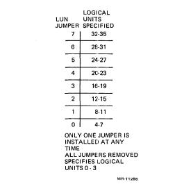
Figure 3-3 RQDX1 Logical Unit Number Jumper Format
