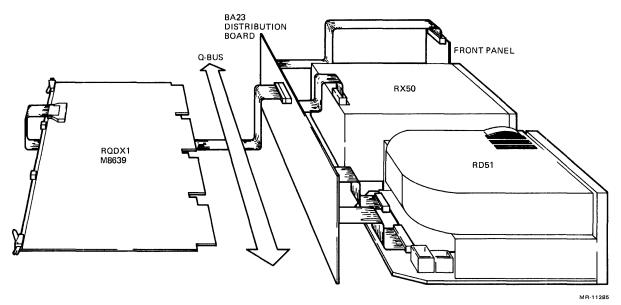
Figure 3-4 RQDX1 MICRO/PDP-11 Signal Distribution Connections
