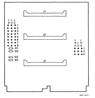
Figure 3-5 RQDX1-E Extender Module Jumper Locations
