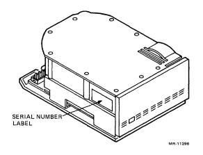
Figure 6-4 RD51 Serial Number Label Location
