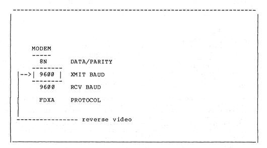
The value of the active parameter changes by means of the up and down arrow keys which cause the parameter to step through its allowable values. The active parameter selection changes by means of the left and right arrow keys. Which moves the active field up and down the list of parameters. 8.1.1.6 PRINTER Field - The printer field displays the parameters for the printer port. The active parameter selection and value changes are the same as for the modem.
