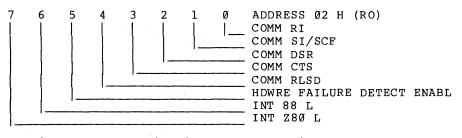
Figure 7. Communications Status Register (8088 Format)
