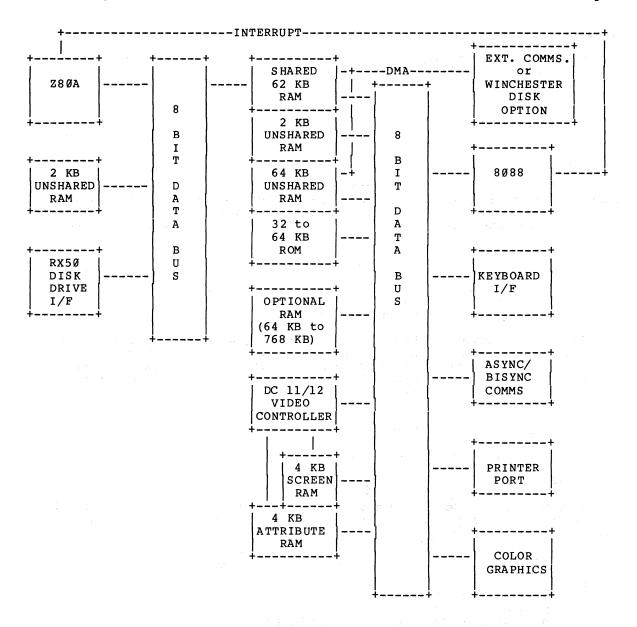
Figure 1. Mother Board Block Diagram
