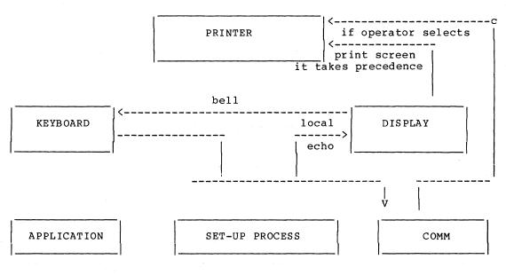
Figure 13. 'Terminal' Mode 'On Line' In 'Printer Controller'
