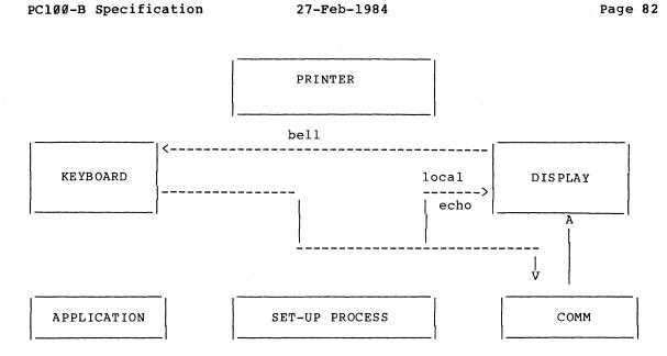
Figure 12. 'Terminal' Mode 'On Line' No Printer Functions
