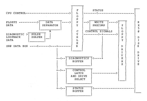
Figure 9. Floppy Controller Block Diagram
