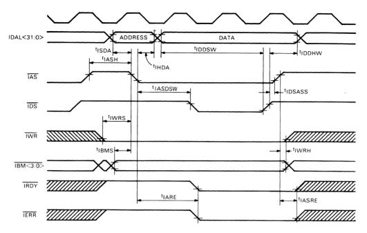
Figure 39 • MicroVAX 78532 I/O Bus Slave Write Cycle Timing
