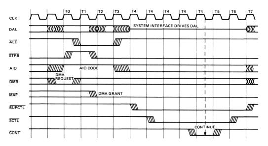
Figure 18 • DCJ11 Stretched Non-I/O Timing Sequence
