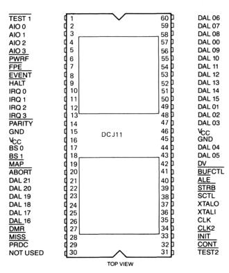
Figure 2 • DCJ11 Pin Assignments
