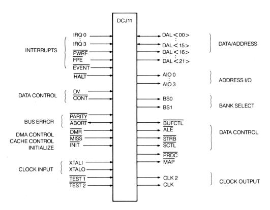
Figure 3 • DCJ11 Signal Functions
