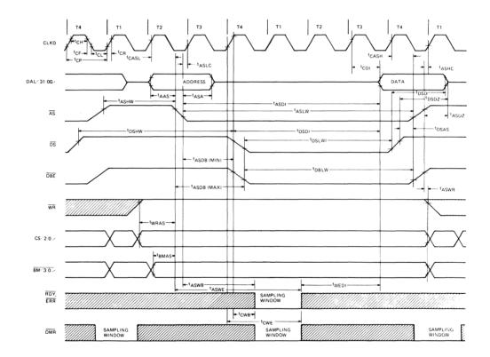
Figure 39 • MicroVAX 78032 CPU Read Cycle Timing Sequence
