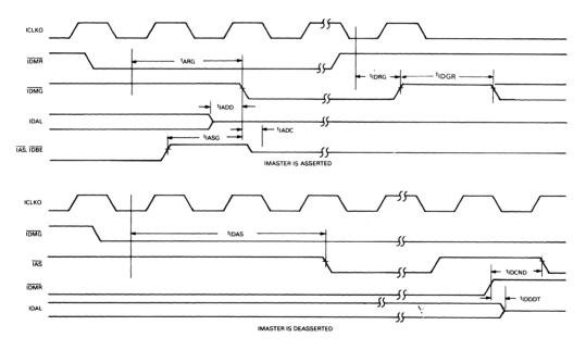
Figure 40 • MicroVAX 78532 I/O Bus DMA Cycle Timing
