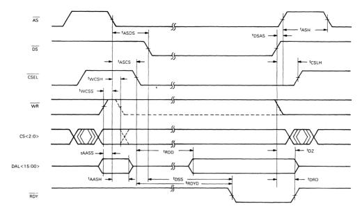
Figure 17 • MicroVAX 78516 Register Read Cycle Timing
