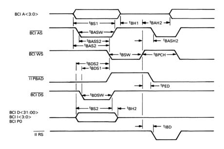
Figure 7 • VAXBI 78743 BCI Bus Interface Write Transaction Timing
