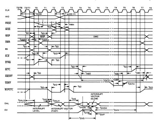
Figure 39 • DCJ11 Interrupt Acknowledge Timing Sequence
