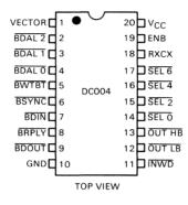
Figure 2 • DC004 Pin Assignments
