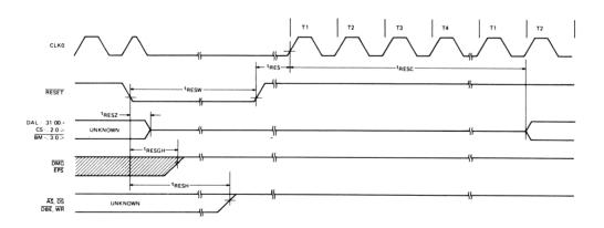
Figure 43 • MicroVAX 78032 Reset Timing Sequence
