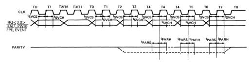
Figure 40 • DCJ11 Interrupt Timing Sequence
