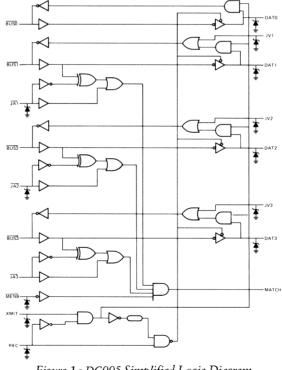
Figure 1 • DC005 Simplified Logic Diagram
