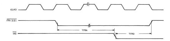
Figure 41 • MicroVAX 78532 I/O Bus Transfer Request Timing
