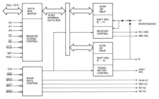
Figure 1 • DC319-AA DLART Block Diagram
