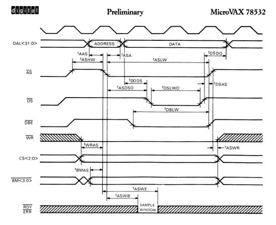
Figure 31 • MicroVAX 78532 MicroVAX Bus Master Write Cycle Timing
