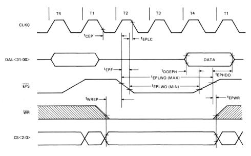
External Processor Write/Command Timing
