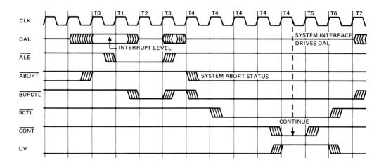
Figure 24 • Interrupt Acknowledge Cycle Timing Sequence
