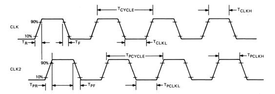
Figure 33 • DCJ11 Clock Output Timing Waveforms
