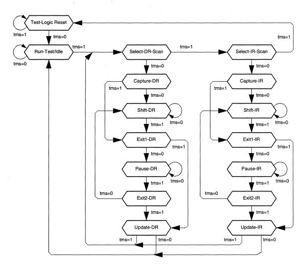
Figure 9: Test Access Port (TAP) Controller State Transitions
