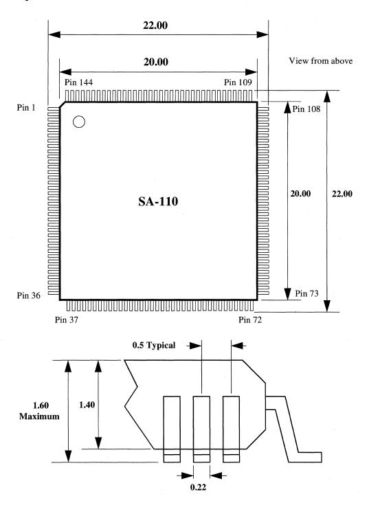
Figure 17: SA-110 144-Pin TQFP Mechanical Dimensions in mm
