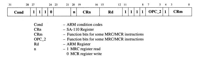
Format of Internal Coprocessor Instructions MRC and MCR
