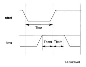
Figure 13: Boundary Scan Reset Timing
