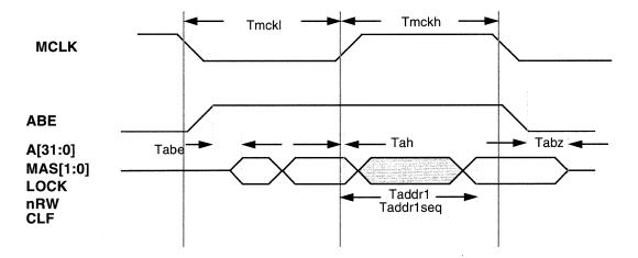
Figure 16: SA-110 Address Timing with APE=HIGH
