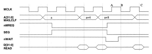
Figure 8: Using nWAIT to Stop the SA-110 for One MCLK Cycle
