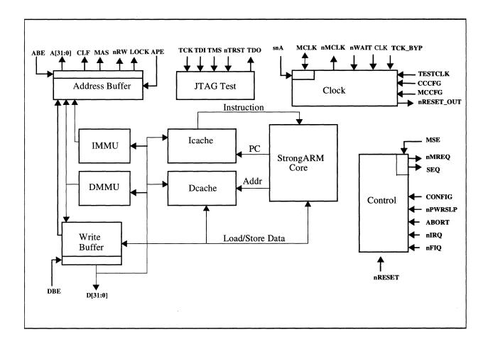
Figure 1: SA-110 Block Diagram
