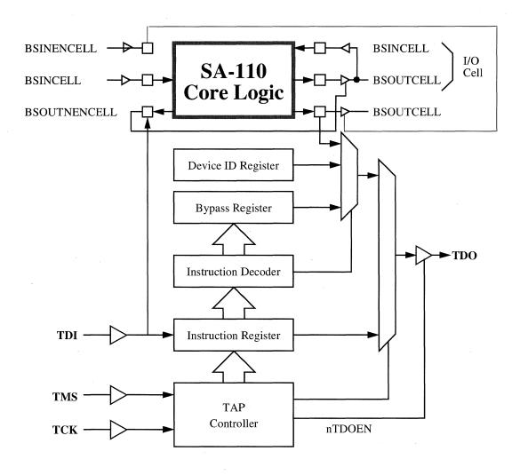
Figure 10: Boundary Scan Block Diagram
