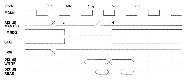
Figure 4: Sequential Read or Write (Two Word)
