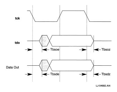
Figure 12: Boundary Scan Tri-state Timing
