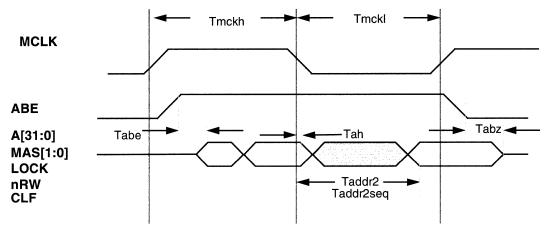
Figure 15: SA-110 Address Timing with APE=Low
