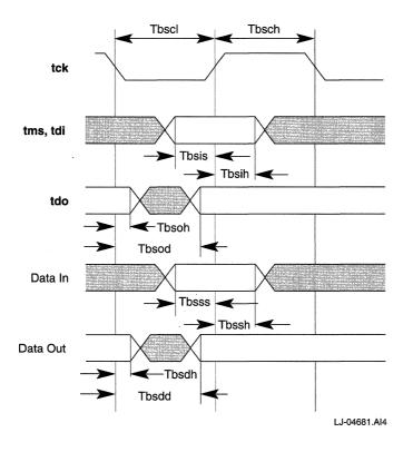
Figure 11: Boundary Scan General Timing
