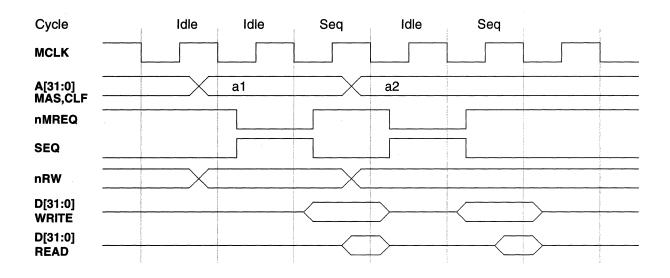
Figure 5: Two 1-Word Nonsequential Reads or Writes Back-to-Back
