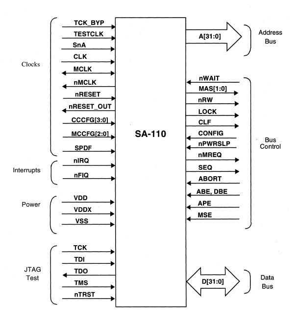
Figure 2: Functional Diagram
