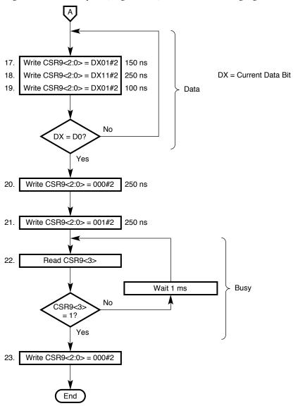
On page 7-7, in Section 7.2.2, **Write Operation**, replace the figure shown in Figure 7-6 Write Cycle (Page 2 of 2) with the following figure:
