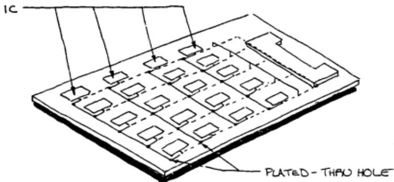
Figure 11 Matrix Type Logic Reference Distribution For Two Sided PC Board
