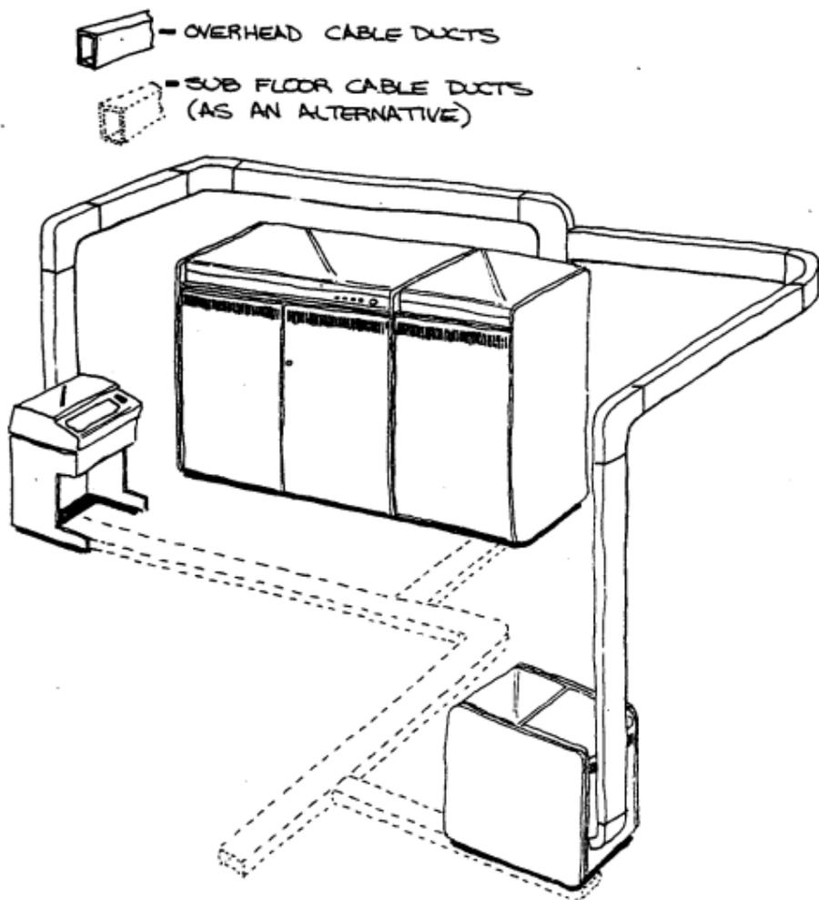
Figure 7 Signal Cable Ducts
