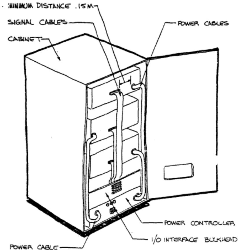
Figure 9 Cabinet Cable Configuration
