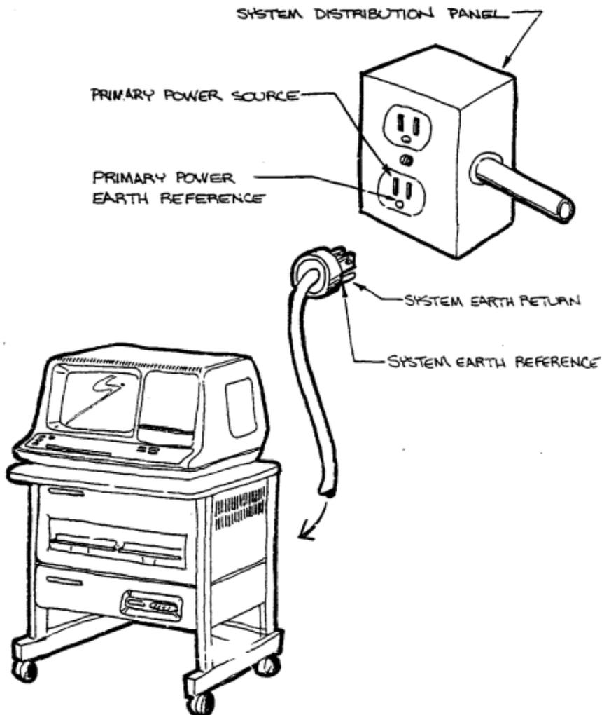
Figure 1 Typical Small Systems Configuration
