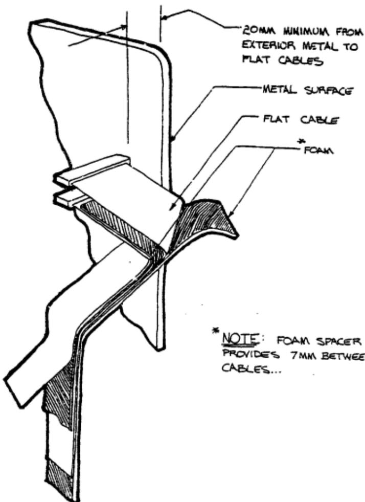
Figure 8 Flat Cable Stacking
