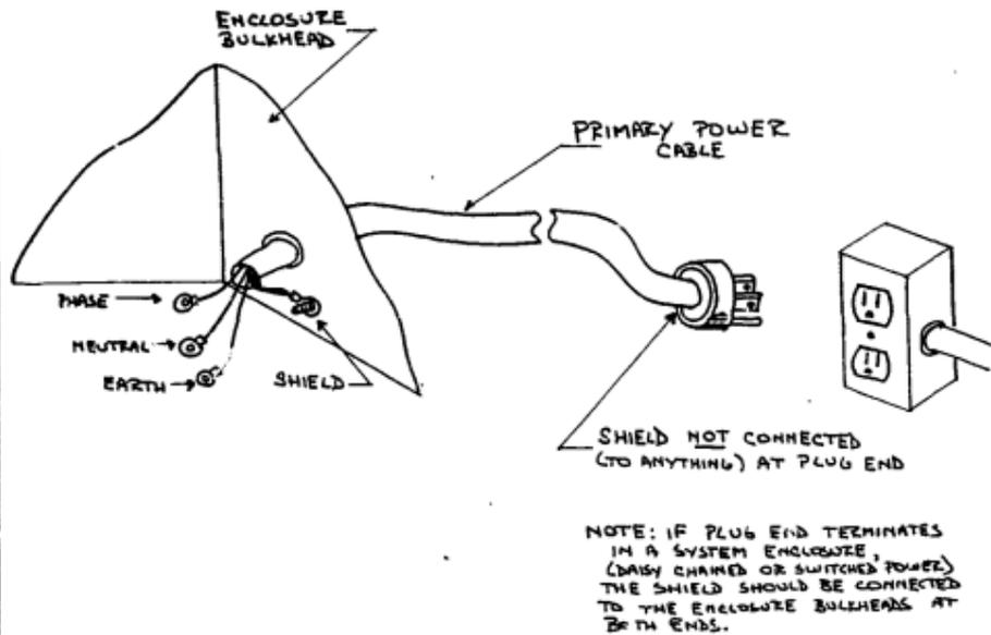
Figure 13 Primary Power Cable Shielding
