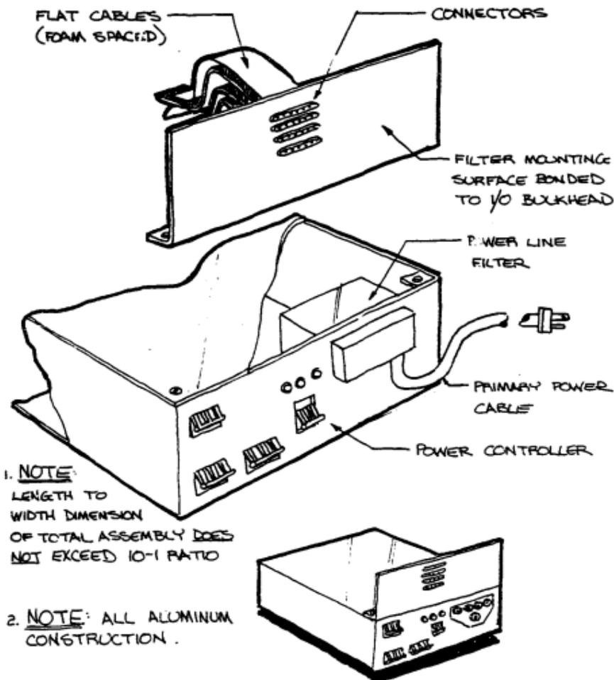
Figure 6 I/O Interface Bulkhead
