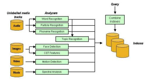
Figure 3: Multiple Analyzers are applied to different multimedia tracks
