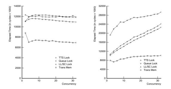
Figure 31: Producer/Consumer Benchmark: Bus and Network
