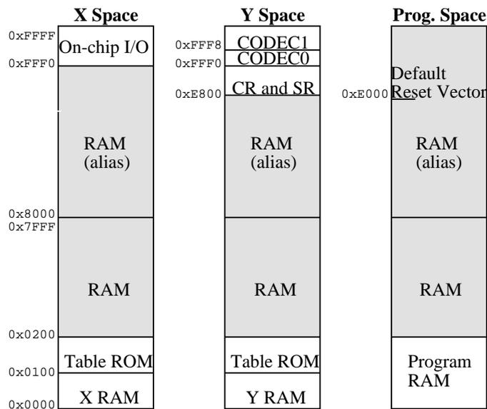
Figure 7: Default normal expanded memory map with data ROMS enabled
