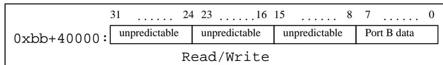
The DSP56001’s host port is a byte-wide read/write data path between the DSP core and an external host [11]. This port is memory mapped into the TURBOchannel I/O space and appears on byte 0 of the TURBOchannel. Read data on the other
