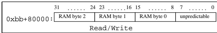
The shared memory size is 32Kx24 bits, with the memory appearing on the upper three bytes on the TURBOchannel data-bus. Read data on the low byte is unpredictable. The shared RAM is indexed by TURBOchannel address bits <16:2>.
