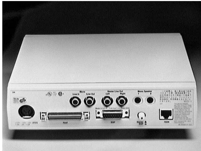
Figure 6: Rear panel of distribution box
