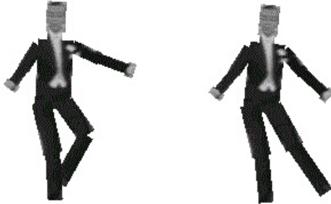
Figure 4: Scaled Prismatic Model with Fred Astaire templates shown in two configurations. Each template can rotate in the image plane and scale along the link direction.
