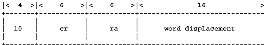
An address is computed by left shifting the displacement field of the instruction by two bits, sign-extending it to 32 bits, and adding register ra. The three low-order bits of the address are ignored (i.e., assumed zero) and register cr of the coprocessor is stored into the 64-bit doubleword at that address. The register address "cr" plus the opcode are transferred to the coprocessors in the ALU pipestage.
