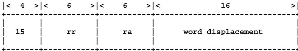
An address is computed by left shifting the displacement field of the instruction by two bits, sign-extending it to 32 bits, and adding register ra. The result is stored in register rr. Note that assignments to the PC take effect after executing the next instruction. Add immediate can be used to synthesize many other instructions, but since the displacement is shifted by two bits it can only add or subtract multiples of four.
