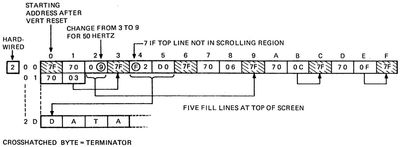
Figure 4-7-6 Fill Line Operation - 50 Hz
