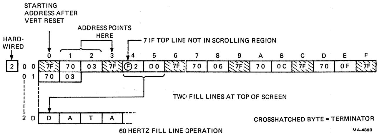
Figure 4-7-5 Fill Line Operation - 60 Hz
