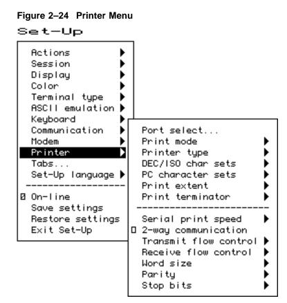
Printer features shown in Figure 2–24 correspond to the control functions listed in Table 2–9. These functions are described in Chapter 5 and Chapter 10.
