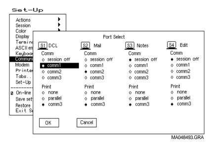
If more than one session is assigned to a single communications port, the Terminal Device/Session Management Protocol (TD/SMP) is used. Pressing the Session key (F4) cycles through each session 1 through 4 in order making it the active session and establishing the corresponding connection as needed.
