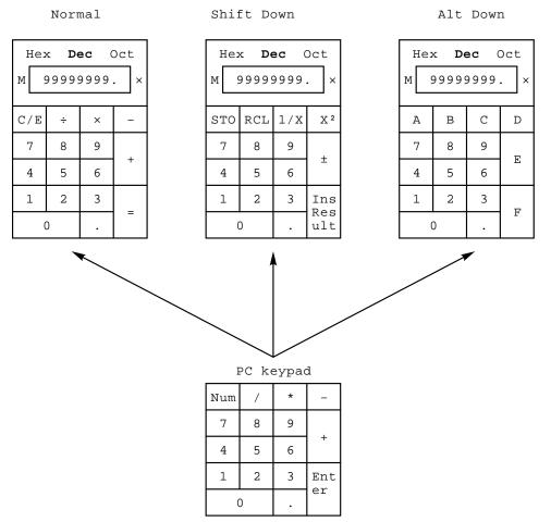
While the calculator is on the screen, all other terminal operations are suspended. The first time the calculator is invoked after the terminal is powered on, the display and memory registers contain 0. The display is eleven characters wide: eight characters are used to display the number's digits, one is used for the decimal point, one for the leading sign bit, and the one in the rightmost position is left blank.
