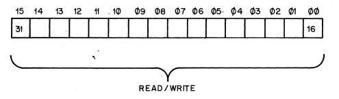
Figure 3-3 Second Data register Out (RG2-DRS)
