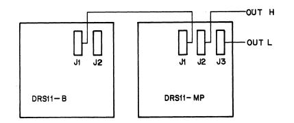
Figure 2-5 DRS11-MP Connected To User Equipment
