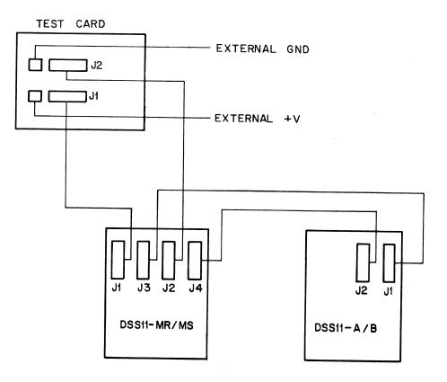
Figure 2-11 Static Pattern Test Cabling
