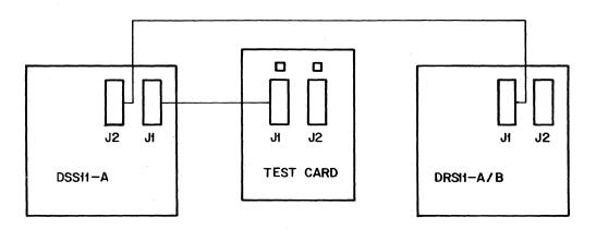
Figure 2-3 DRS11-A/B Looped With DSS11-A
