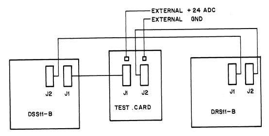
Figure 2-4 DRS11-B Looped With DSS11-B
