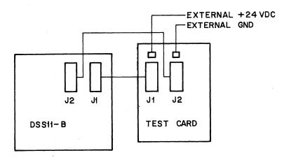
Figure 2-2 DSS11-B Stand Alone Test 6
