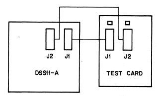
Figure 2-1 DSS11-A Stand Alone Test 6
