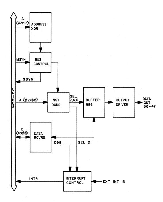
Figure 4-1 DRS11-A/B Block Diagram
