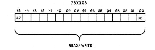
Figure 3-4 Third Data Register Out (RG3-DRS)
