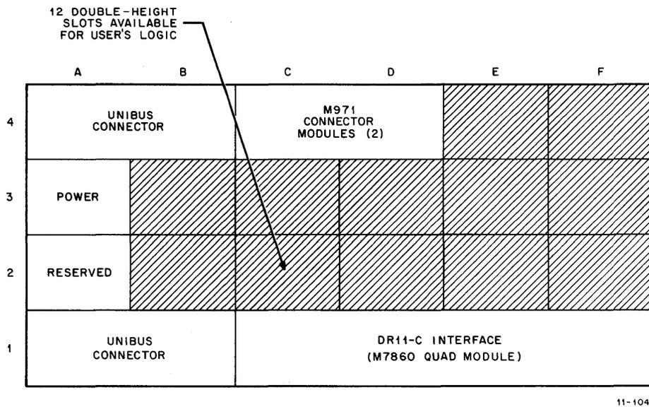
Figure B-1 DR11-C Mounted in BB11 System Unit
