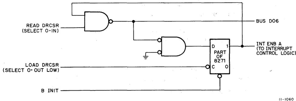
Figure 4-5 Status Register Input/Output Gating (one bit position)
