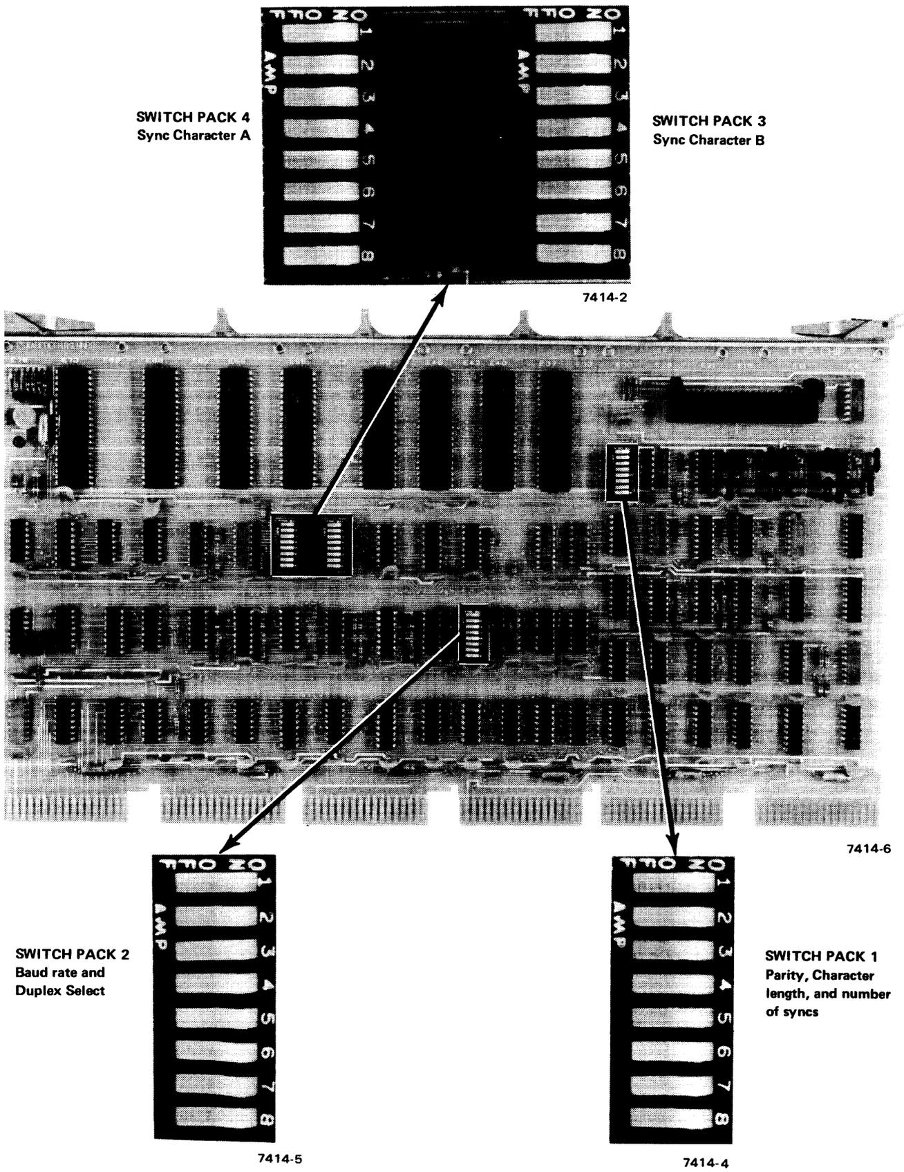
Figure 2-6 Location of Sync Switches on M7839 Module
