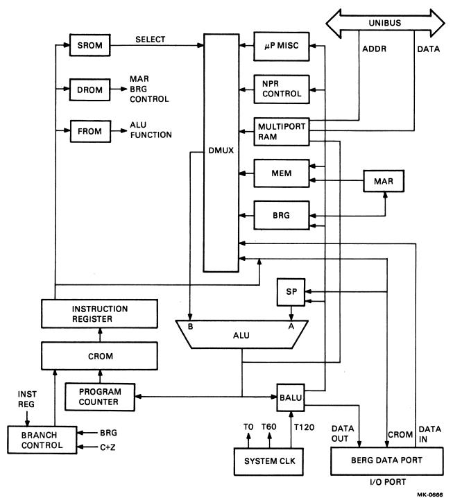
Figure 1-1 Microprocessor Simplified Block Diagram
