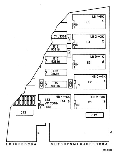
Figure 3-1 Extract of M8207 Module Component Layout
