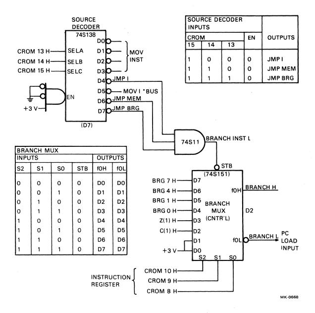
Figure 2-13 Branch Control Logic
