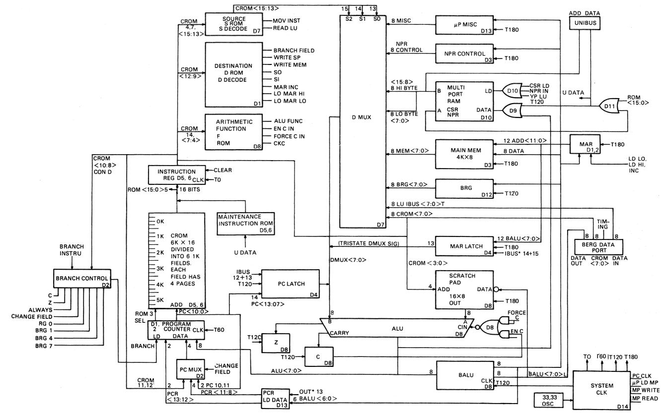
Figure 2-1 Microprocessor (Sheet 1 of 3) a. Interconnection Between Controlling Elements
