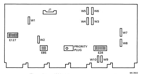
Figure C-1 M8207 Microprocessor Jumper Locations
