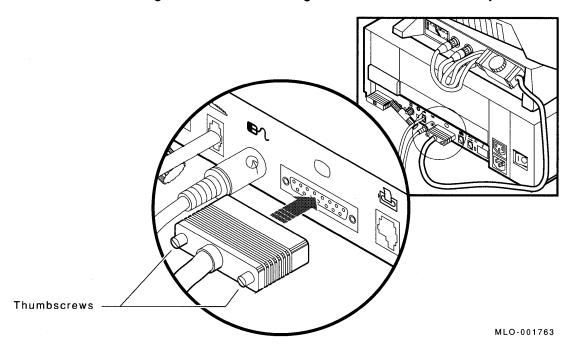
Tighten the thumbscrews on the monitor connector by turning them to the right.
