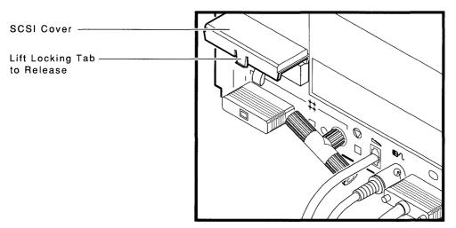
To remove the SCSI terminator, place your fingers under the loop attached to the terminator and pull out. Figure 4-2 shows you how to remove the terminator.
