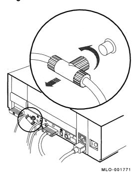
Check that you have not disconnected a terminator from an active ThinWire segment. This procedure disrupts network operation.
