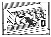
Remove the tape cartridge and store it in its plastic container.
