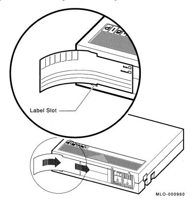
Figure 3-5 Labeling a Tape Cartridge
