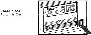
Release the load/unload button to the out (unload) position. The red and green lights flash slowly as the tape rewinds. When the tape is completely unloaded, the red light goes off and the green light comes on.
