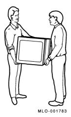
Always repack the system unit in its original packing material when moving or relocating your VAXstation 3100 Model 40. This precaution will protect the hard disks from damage.
