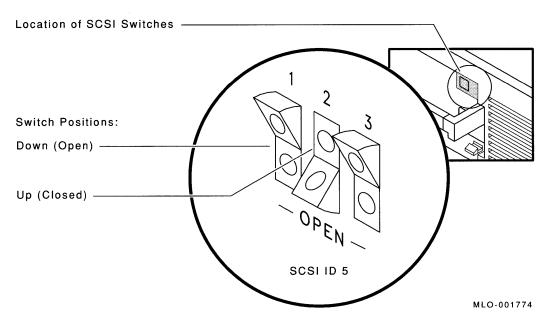
The TK50Z tape drive is shipped from the factory with the switches set to SCSI ID 5. The switches should be in the following positions (left to right): down, up, down. Leave the switches in the default (factory) position.
