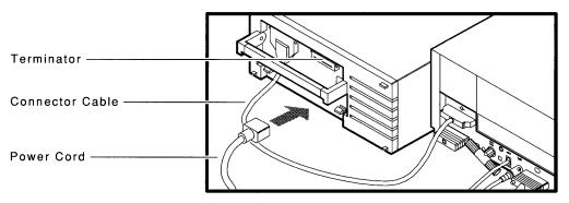
Figure 4–6 Connecting One RRD40 Expansion Box
