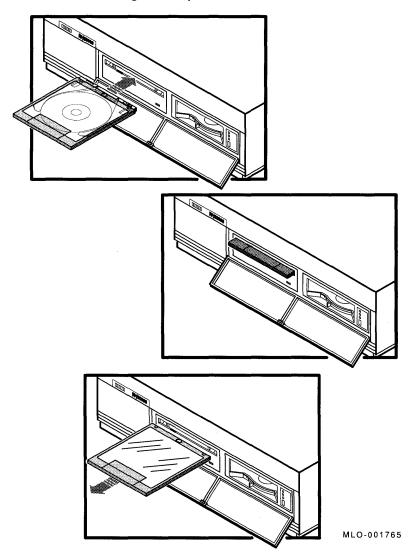
Slide the caddy in as far as it will go and then remove it. When it is removed, you will notice that the disc and its housing remain in the drive. Only the transparent sleeve comes out.
