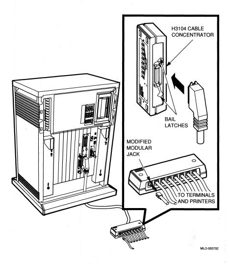
5. If you have not already done so, connect the remote terminal or printer to the other end of the cable. Your terminal or printer documentation shows how to connect the cable. If the printer or terminal does not have a modified modular jack connection, use a passive adapter (H8571-A), available in 25- and 9-pin models.
