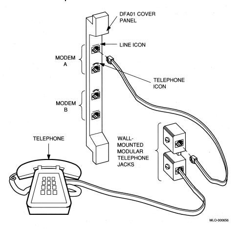
The following describes an alternative method of installing voice communication on the DFA01 modem. The telephone is connected to the DFA01 cover panel, which is, in turn, connected to the wall-mounted modular telephone jack (see Figure 14).
