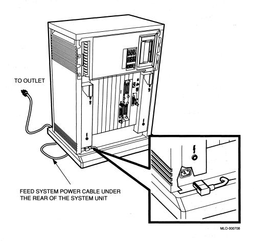
5. Plug the pronged end of the power cable into the wall outlet.
