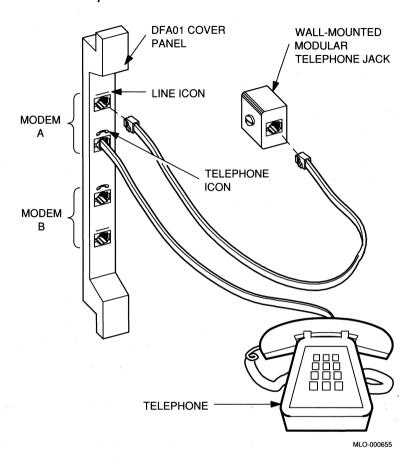
If you do not plan to use modem B, do not perform the following step. If you require use of a second modem, set up modem B for use by continuing with step 5.
