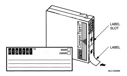
To indicate that the tape was recorded on a TK70 tape drive, check the box labeled 296MB. The 95MB box is used for tapes recorded on a TK50 drive.
