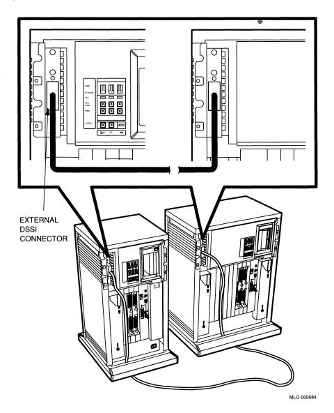
If one of the KA640 CPU modules fail, all satellite nodes booted through that KA640 lose connections to the system disk. Each satellite node knows, however, that the system disk is also available through a second path—that of the remaining KA640 module. The satellite nodes establish a new connection through the other system and continue operation.
