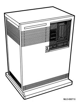
The front panel has a sliding window controlled by a 3-position rotary lock. You can lock the window in one of three positions: closed, partially open, and fully open. Each position limits access to certain system controls. When the window is locked in any of its three positions, you can still raise it to a higher position. However, you cannot lower it beyond the locked position without using the key.
