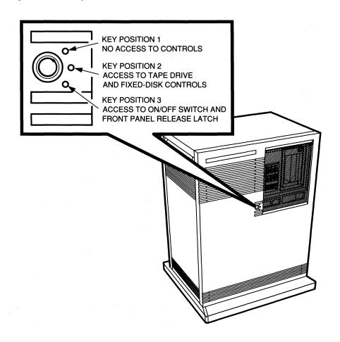
When the window is up and the key is turned to position 1, the window is locked in the closed position. You cannot use any controls when the window is closed, but lights indicating power to the system and activity on the disks and tape are visible through the window. Figure 1–3 shows the closed window and key position.
