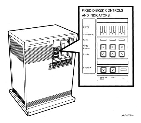
The system has controls and indicators for three RF30 fixed-disk drives. Each RF30 has the following controls and indicators arranged in a column on the control panel.
