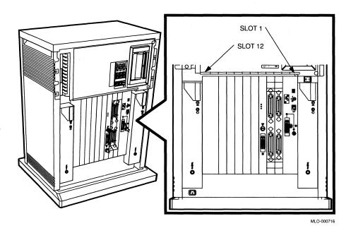
The number and type of modules installed in your system depend on your configuration. Each slot, even an empty one, is protected by a module cover panel. Together the panels form a shield with a two-fold purpose: to protect external devices from electrical interference generated by the system, and to protect the system from electrical interference generated by external devices.
