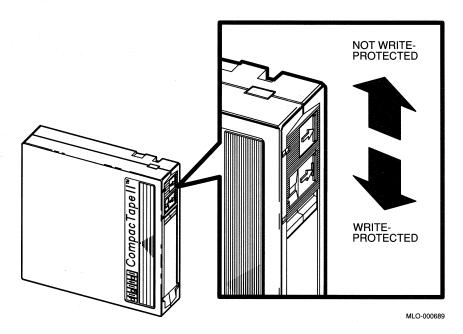
When you insert a write-protected cartridge into the drive, the orange indicator light comes on. The system recognizes the tape as being writeprotected under any one of the following conditions:
