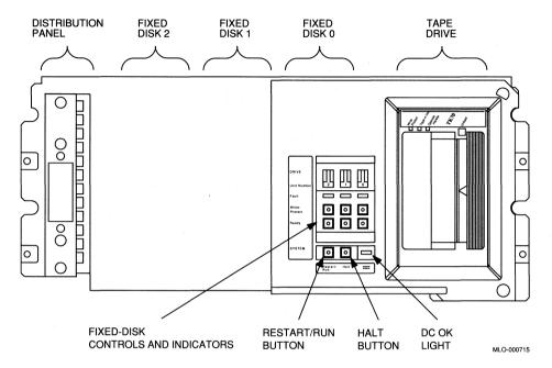
The RF30 control panel has several buttons and indicators for each of the three possible drives. When you turn on your system, indicator lights come on for each drive present. Chapter 3 describes how to use the control panel.
