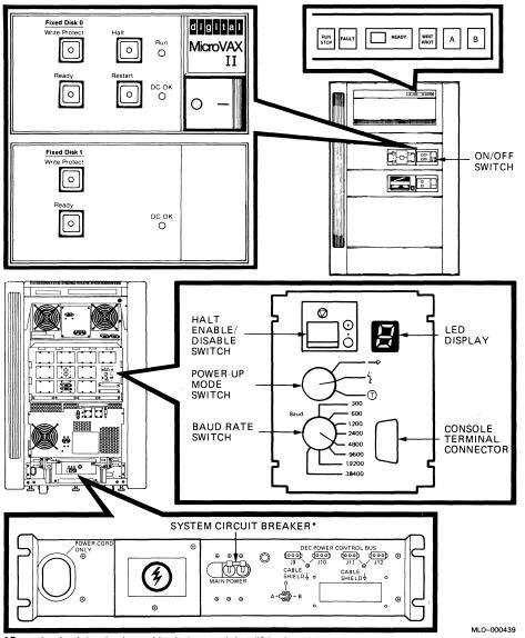
\*Reset the circuit breaker by pushing it down and then lifting it to the up position.
