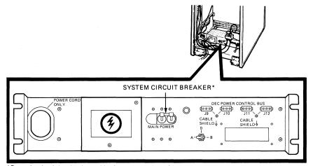
\*Reset the circuit breaker by pushing it down and then lifting it to the up position.
