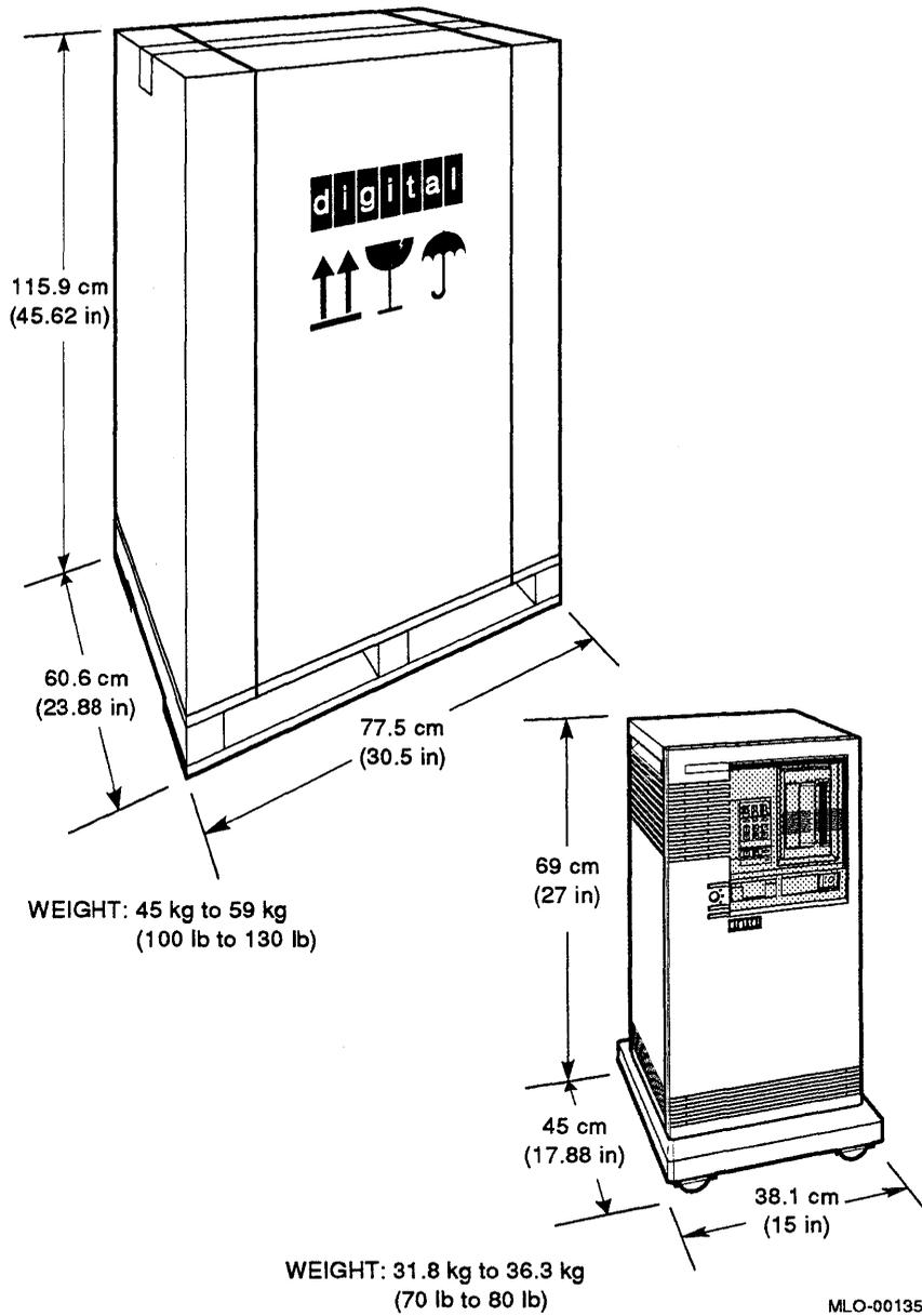
**Figure 2-4: B213F Expander and Shipping Container Dimensions**
