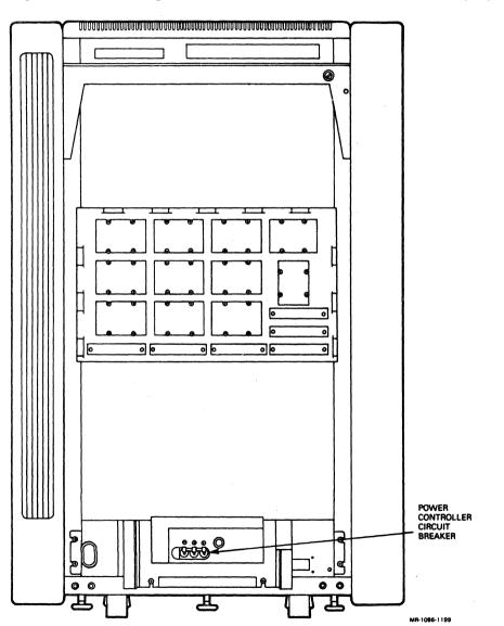
Figure 2-42: Setting the Power Controller Circuit Breaker to 1 (On)
