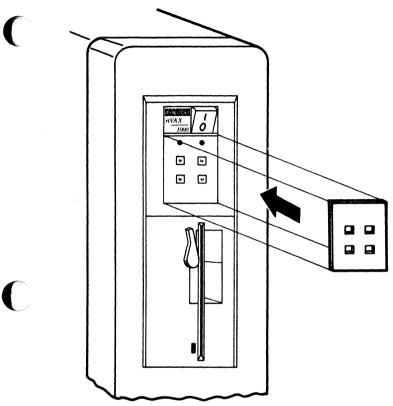
Figure 2-18: Labeling the Control Panel on the Pedestal Model
