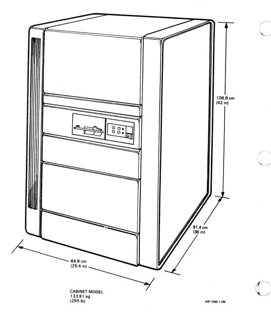
Figure 1-3: Physical Specifications for the Cabinet Model
