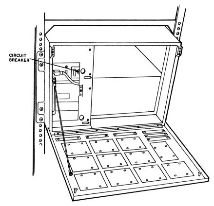
Figure 5-2: Checking the Circuit Breaker on the Cabinet Model
