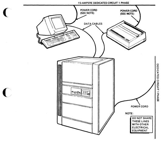
Figure 2–2: System Power Considerations for the Cabinet Model
