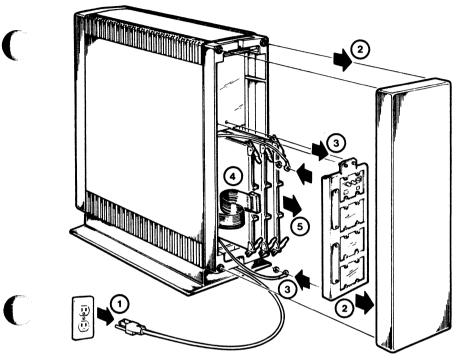
Figure 3-18: Module Removal and Replacement
