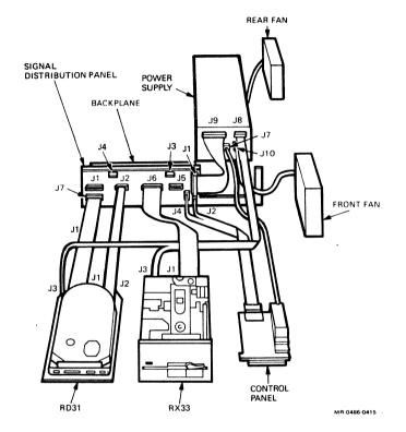
Figure 3–12: BA23-A Internal Cabling
