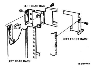
Figure 2-8: Securing the Mounting Rails
