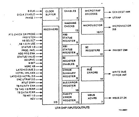
\*Note: Some signals are sent to UTR chip even if memory management is not enabled, but are not checked unless "TB Parity Enable H" is sent from ADK.
