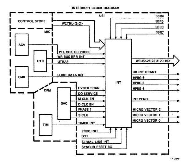
Figure 16-3 Interrupt Block Diagram
