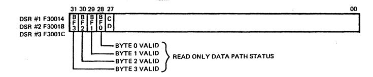
NOTE 1: THERE ARE FIVE FLAGS THAT KEEP TRACK OF THE DATA IN THE DATA BUFFER, NAMED CD AND BF3 THROUGH BF0. IF CD = 1, THEN THE BUFFER HAS FOUR BYTES OF DATA FROM THE CMI AND BF3 THROUGH BF0 ARE ALWAYS 0. IF CD = 0, THEN BF3 THROUGH BF0 INDICATE WHICH BYTES IN THE DATA BUFFER HAVE VALID UNIBUS DATA. IF THEY ARE ALL 0, THEN THE BUFFER IS CONSIDERED EMPTY.
