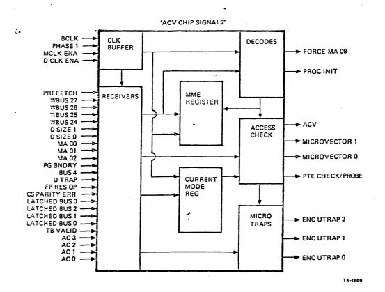
Figure 11-11 ACV Chip Signals Input/Output
