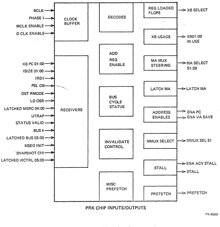
Figure 13-6 PRK Chip Signals Input/Output
