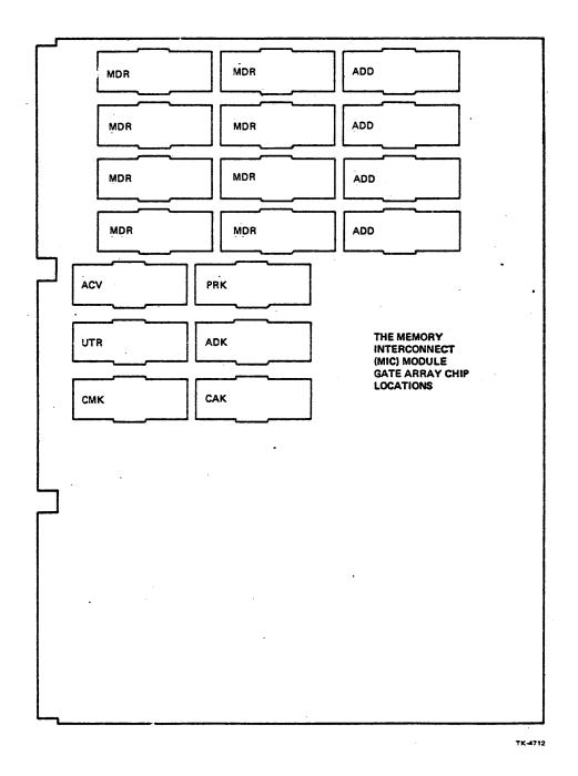
Figure 4-2 MIC Gate Array Locations
