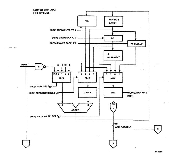
Figure 10-2 Address Chip 4 X 8 Size and Signals
