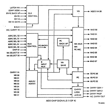
Figure 10-3 Address Chip Signals In/Out
