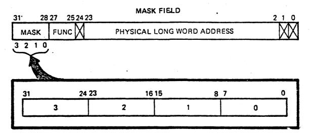
EACH BIT IN THE MASK FIELD CORRESPONDS TO A PARTICULAR BYTE IN SUBSEQUENTLY TRANSFERRED DATA FORMAT. THESE BITS SPECIFY WHICH OF THE CORRESPONDING DATA BYTES ARE TO BE READ OR WRITTEN. THE BYTE IS SELECTED WHEN THE MASK BIT IS SET.
