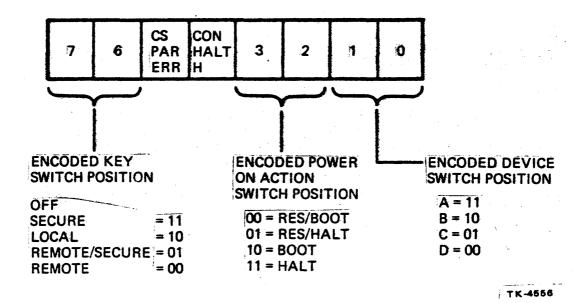
Figure 6-4 Front Panel Status Register F820
