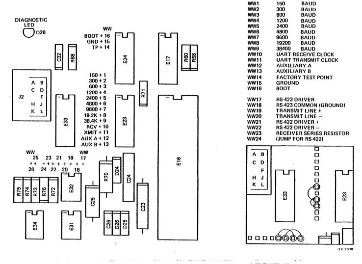
Figure 18-3 Interface Selection Jumper Locations
