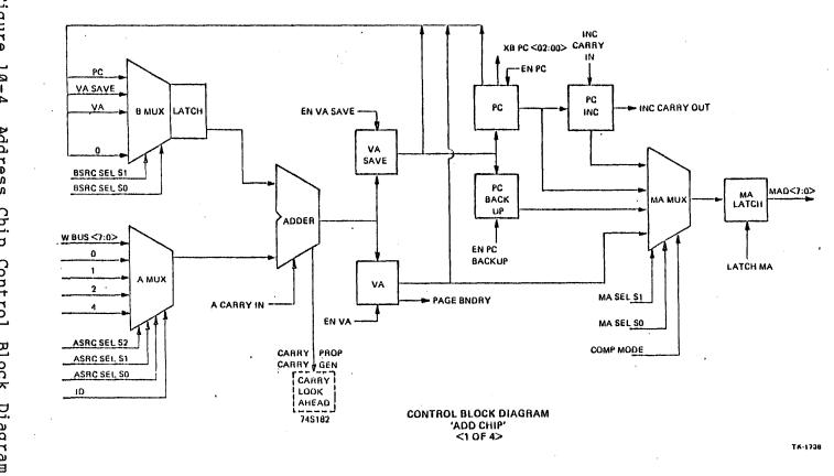
Figure 10 - 4Address Chi p Control Block Diagram
