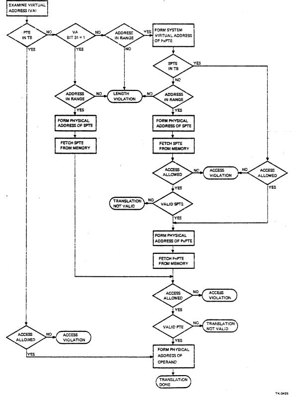
Figure 9-13 Address Translation Faults
