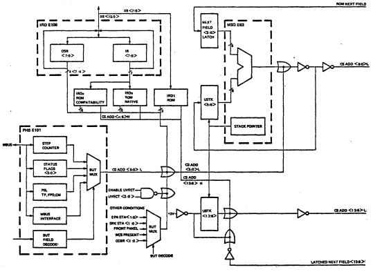
LEI CHIP FUNCTIONAL SCHEMATIC COMET MICROSEQUENCER,
