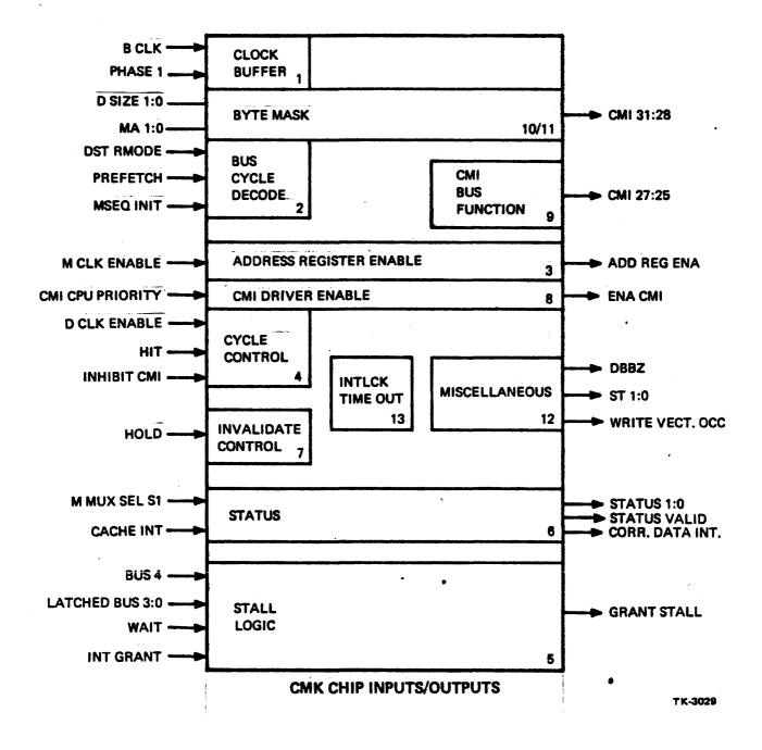
Figure 14-6 CMK Chip Inputs/Outputs
