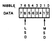
IN ORDER TO PERFORM AN ARITHMETIC FUNCTION ON TWO SUCH STRINGS (ADD), THE CARRY FROM NIBBLE 6 WOULD HAVE TO BE PROPAGATED TO NIBBLE 7, AND NIBBLE 7 PROPAGATED TO NIBBLE 4, AND SO ON.....
