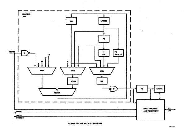
Figure 10-1 Simplified Chip Block Diagram
