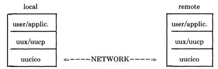
At the highest logical level is the user or application program. This level will use uux or uucp to initiate requests for file transfers and/or remote job execution. uux is the remote execution program and uucp is the program that spools user requests for file transfers. Both programs convert higher level requests into the format required by the file transfer daemon uucico. Each request is queued in the appropriate spool directory.
