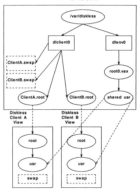
Figure 1-2: Client Views of the Diskless Server Area
