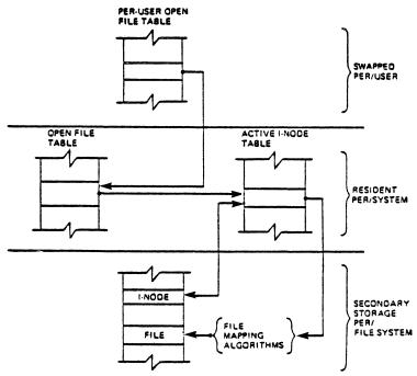
Fig. 2 File system data structure.
