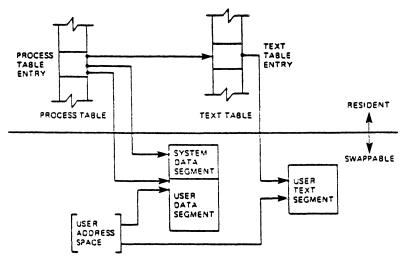
Fig. 1 Process control data structure.
