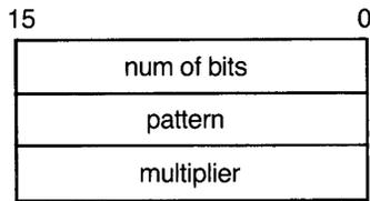
**pattern-state.** A two-word block containing a pattern position and multiplier count. Passed by reference. These two words are updated after the curve is drawn if updating is specified with the pattern-action parameter.
