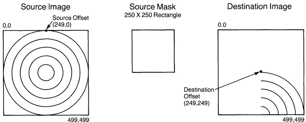
**Figure 2-1. Source Offset and Destination Offset**
