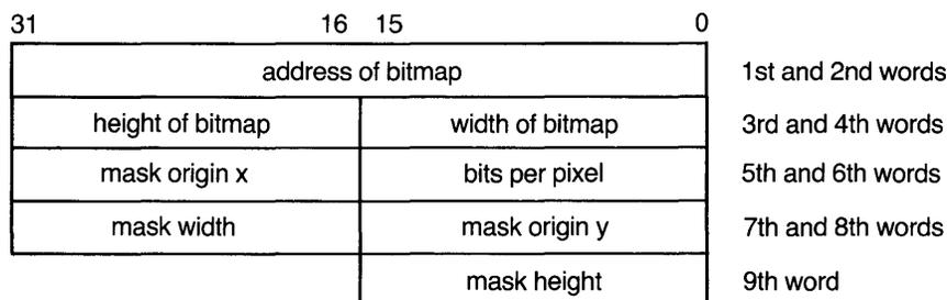
If the mask is a virtual display, the mask parameter is a block with the following format:
