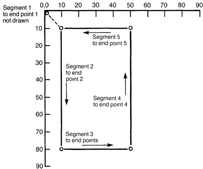
**Figure 3–1. Drawing a Curve**
