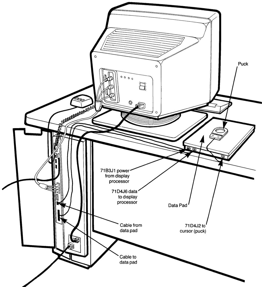
**Figure 21. Connecting the Data Pad**
