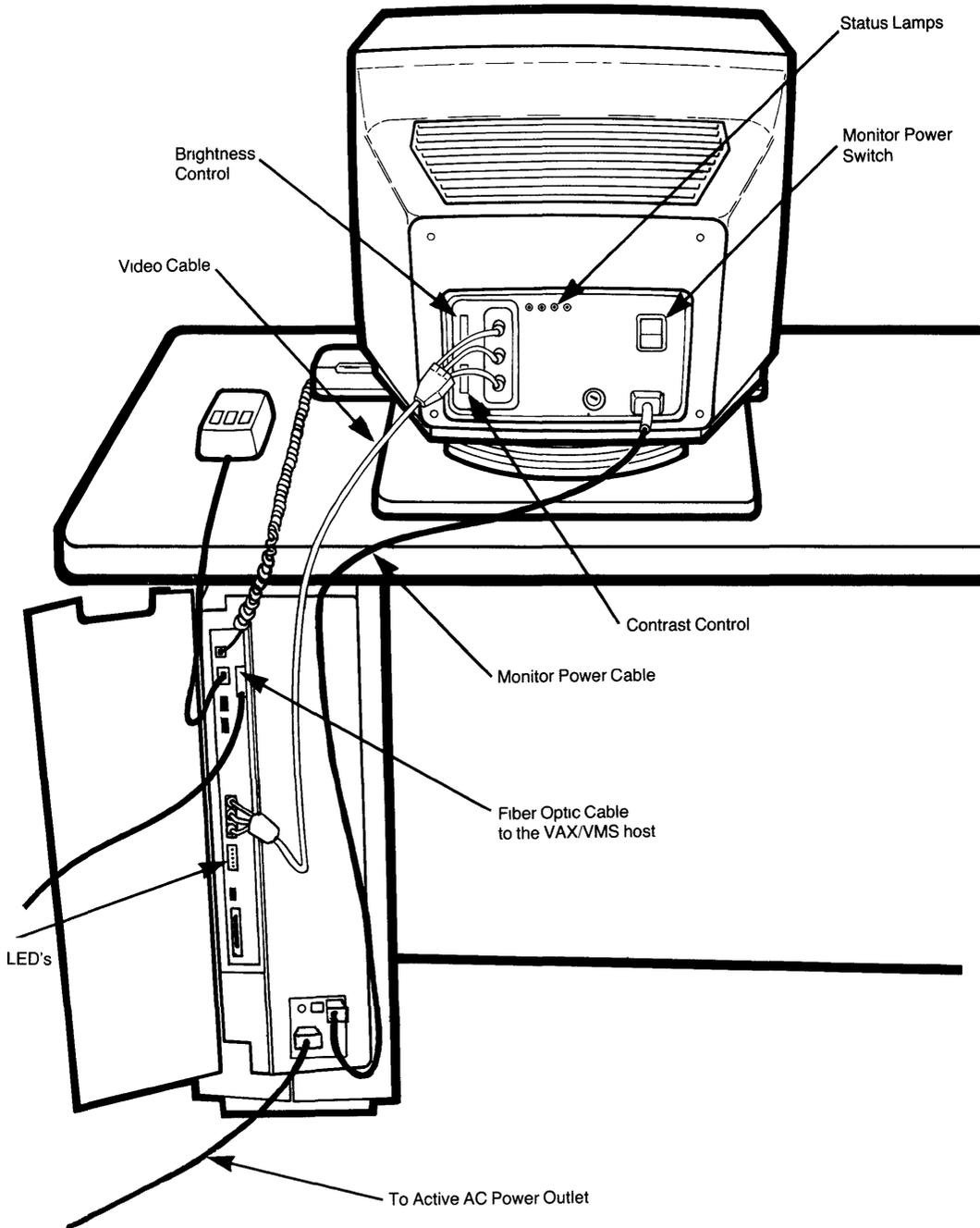
**Figure 2. The VAXstation 100 (Rear View)**
