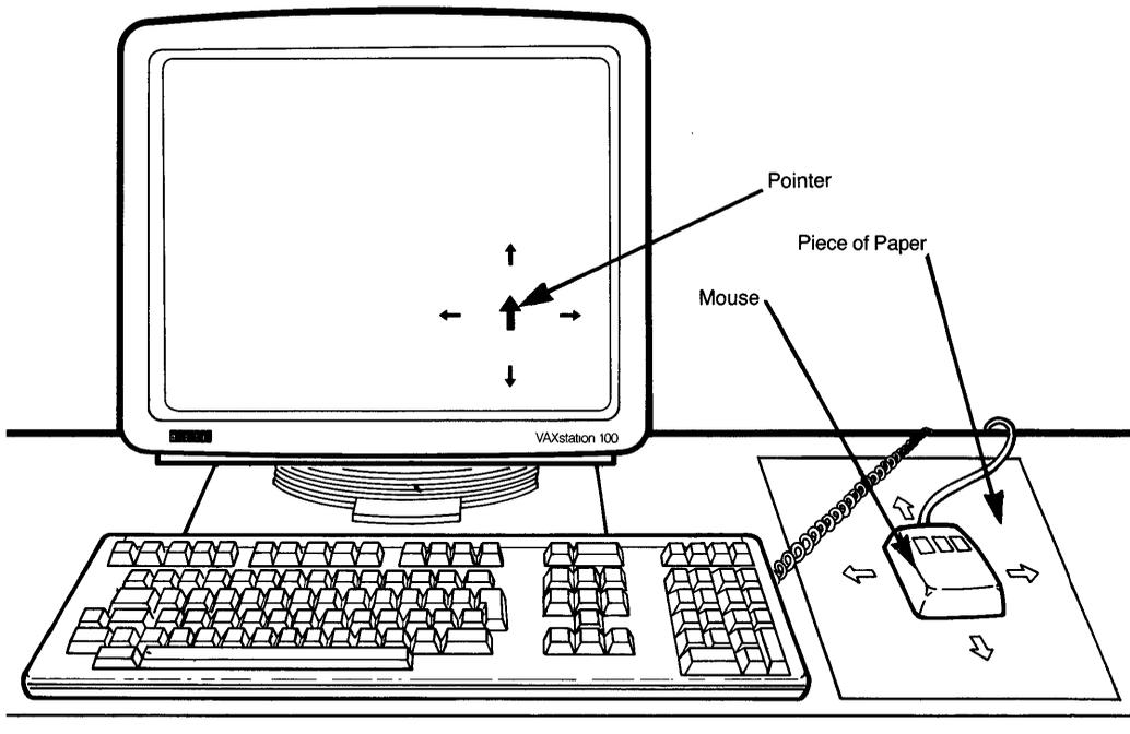
**Figure 6. The *Mouse* and the *Pointer***
