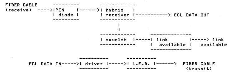
the FOT/R has four sections. These are: 1. the hybrid receiver, 2. the squelch circuit, 3. the link available circuit and 4. the transmit L.E.D. driver.
