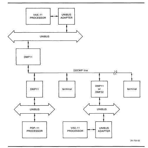
Figure 2–1 Typical DMP11/DMF32 Multipoint Configuration
