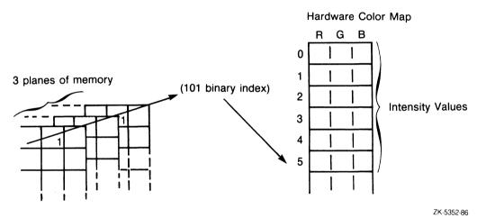
If your application is not using the UIS environment, it must load any values it uses into the hardware color map. To load values into the hardware color map, use the Set Color Map Entries QIO; specifying an index into the color map at which to begin initializing, the address of the buffer containing the desired intensity values, and the length of the buffer. You may call this QIO at any time to redefine the values in the color map.
