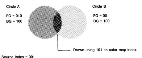
When objects are written to the screen, the system performs a logical operation on the present contents of the screen bitmap and the source index. The logical operation is determined by the specified writing mode. Because the DSO mode was specified in Figure 5–1, Circle A's foreground index 010 is ORed with the source index, 001, resulting in the number 011.
