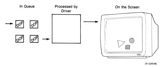
At any given time, the driver may be processing a number of DOPs. To synchronize activity, you must manipulate the queue *and* be aware of whether the driver is currently processing DOPs.
