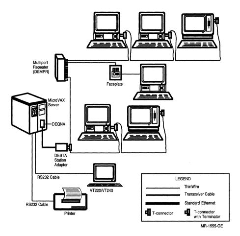
Figure 4–4 Daisy-Chain Configuration with DEMPR
