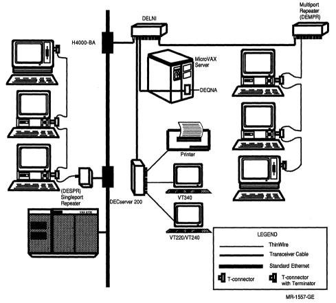
Figure 4-6 Daisy-Chain with DECserver 200 and DESPR
