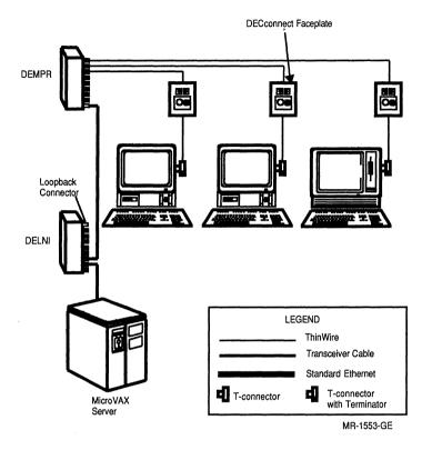
Figure 4–2 DECconnect Faceplate with DELNI Configuration
