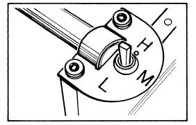
Using "HIGH" for single sheet printing may cause premature wear on printwheels.
