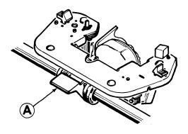
With the Model 630, the platen position or paper thickness adjustment and the print intensity or hammer energy switch are a combined function.
