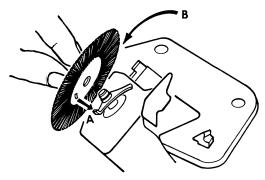
The printwheel should be handled only by the center hub and be installed or removed from the printer in a straight motion.
