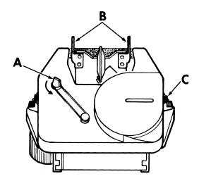
With the carriage in closed position, tighten the exposed ribbon by turning capstan "A" in the direction indicated; push back ribbon latches "C", and install cartridge, ensuring that the ribbon slips tautly over the ribbon guides "B"; release the latches, ensuring that they are firmly positioned over the cartridge lips; retighten the ribbon. Ensure that the ribbon does not bend or fold exiting or reentering the cartridge.
