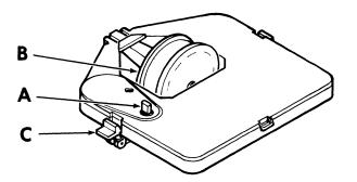
Remove ribbon slack by turning the knob "A" counterclockwise.
