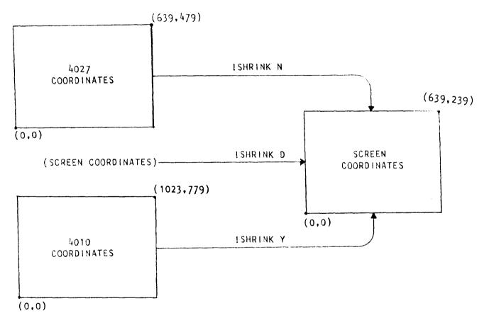
Figure 4-1. Coordinate Scaling
