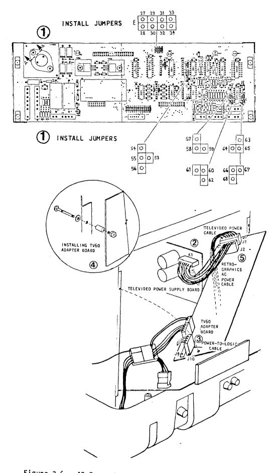
Figure 2-6. AC Power Connections and TV60 Adapter Board Installation
