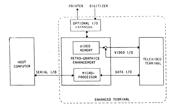
Figure 1-3. Retro-Graphics Functional Block Diagram
