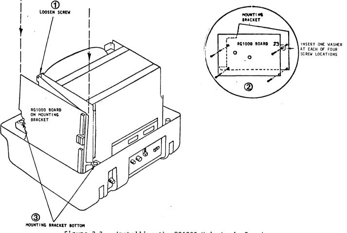
Figure 2-3. Installing the RG1000 Main Logic Board
