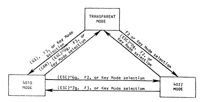
Figure 1-2. Mode Transition Diagram
