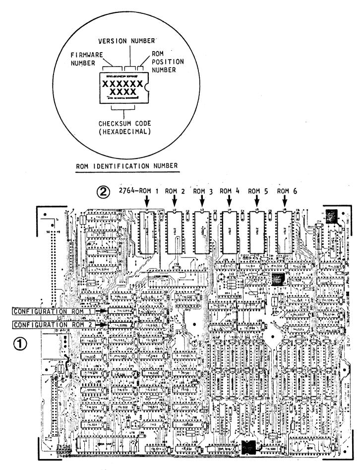
Figure 2-2. Installing the RG1000 Firmware
