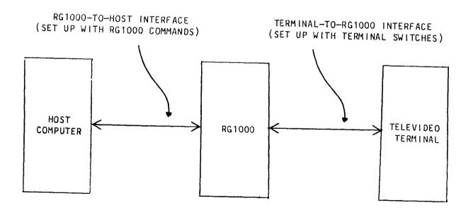
Figure 2-1. Terminal/RG1000 Interfaces
