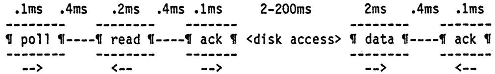
The time delay between messages is needed so that the sender of a message has time to execute the necessary code to receive an answer-back message. In order to minimize this time delay, a sophisticated disk buffering scheme is used in the network master, so a typical transaction is completed in fewer than 10 ms.
