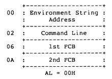
Figure 7-7. EXEC Load and Execute Parameter Block
