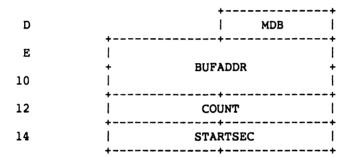
Figure 9-4. Input and Output Parameter Block
