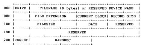
Figure 7-2. DOS Standard File Control Block
