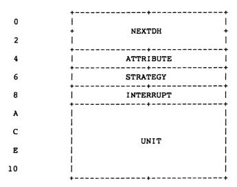
Figure 9-1. DOS Device Header
