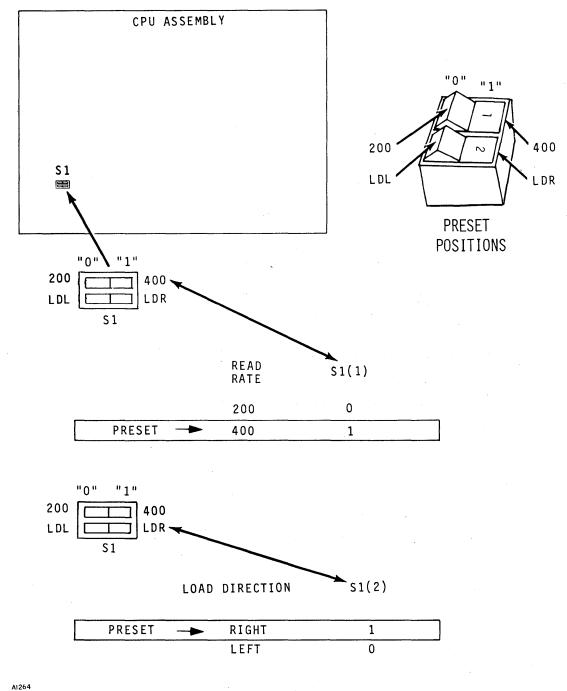
Figure 4-3. CPU Switch Settings.
