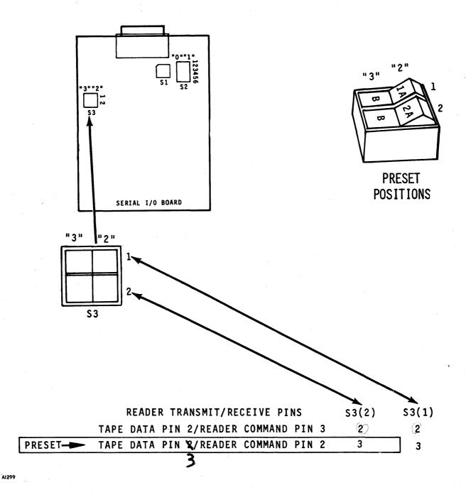
Figure 5-11. I/O Switch Settings - S3.
