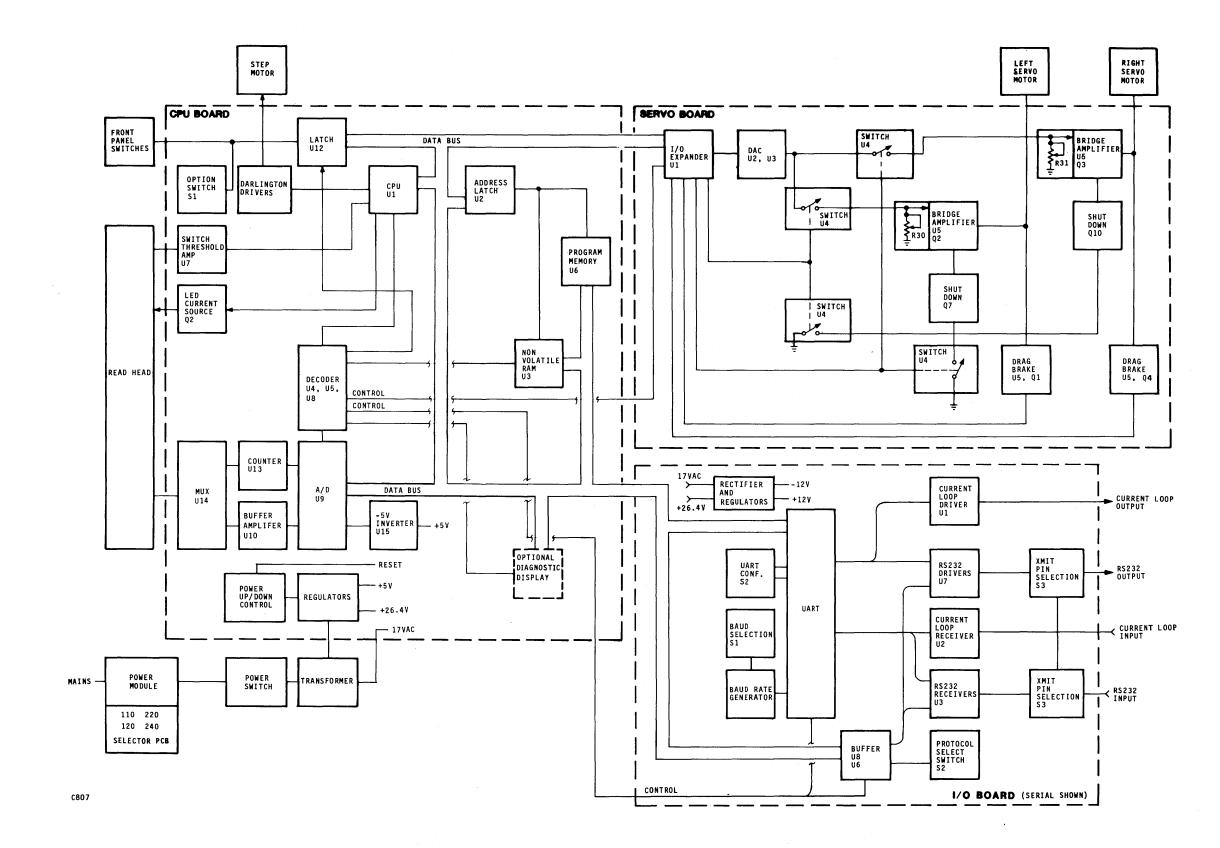
Figure 7-3. Tape Reader Block Diagram (Serial I/O).
