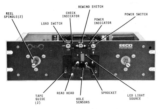
A1257 Figure 6-1. Front Panel Controls and Indicators.
