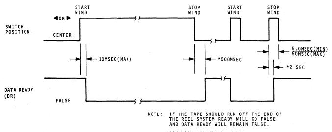
\*CAN VARY DUE TO REEL SIZE AND TAPE LOADING.
