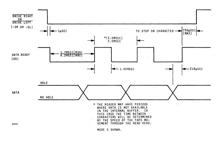
Figure 4-5. Slew Timing.
