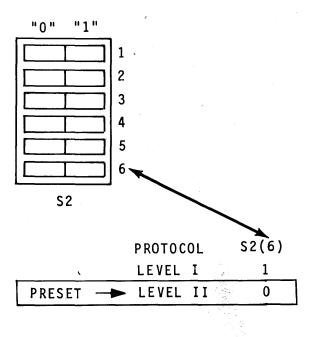
Figure 5-10. Data Configuration Switch Settings - S2.
