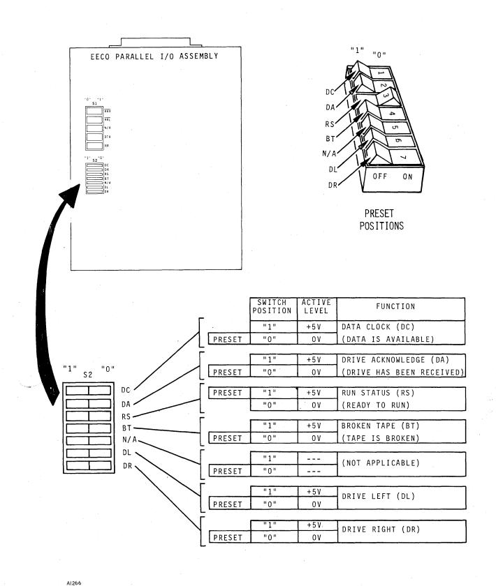
Figure 3-5. I/O Switch Settings - S2.
