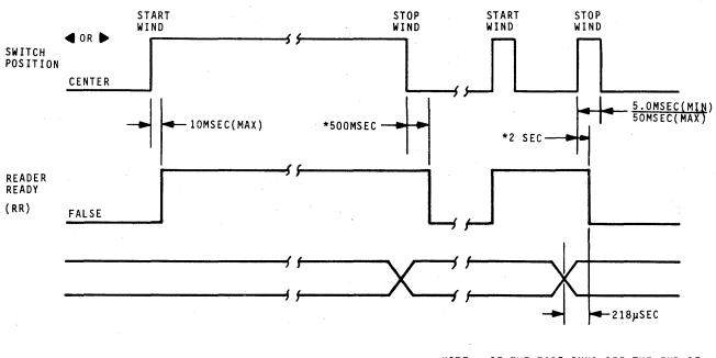
NOTE: IF THE TAPE RUNS OFF THE END OF THE REEL A BROKEN TAPE SIGNAL WILL BE ISSUED, READER READY WILL STAY FALSE.
