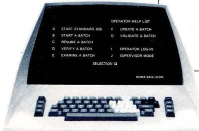
With System 480, data is edited and checked as it is keyed—and not at the end of a batch. Using features like range checking and table lookup. Multiple check digit validation. Mandatory entry and field boundary checks. Crossfooting and more. Just about any edit function you can imagine.
