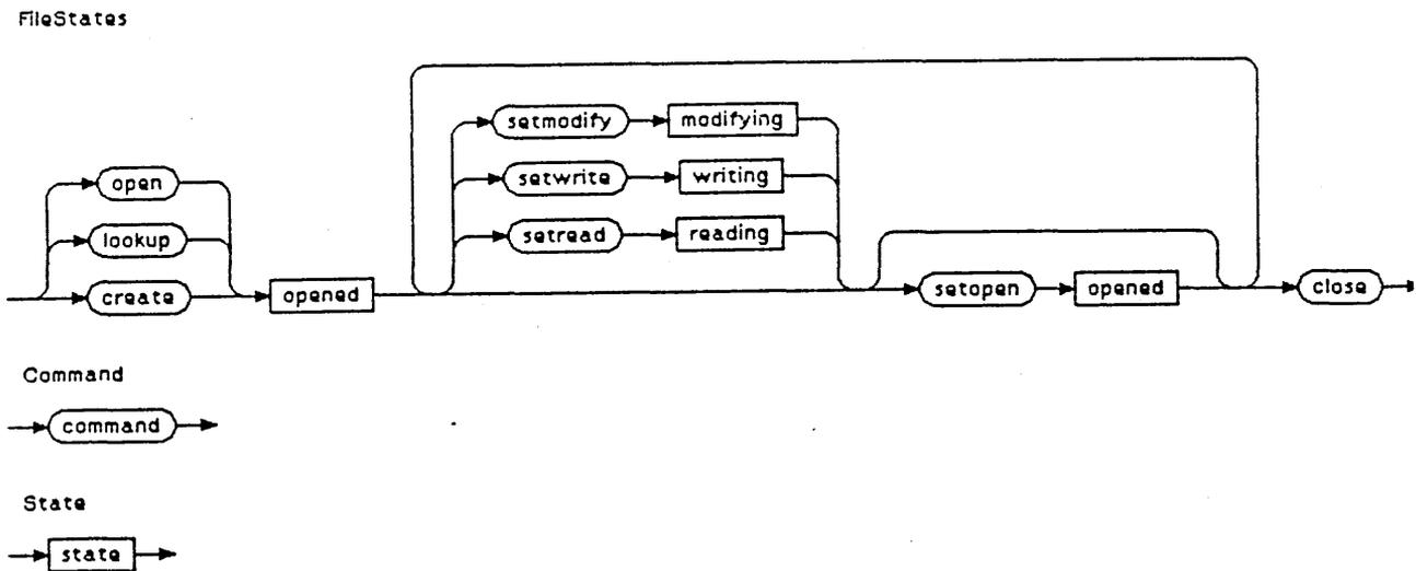
This figure shows how the I/O state of a file is changed when different commands are executed. Commands not shown in the figure do not affect the I/O state of a file. Whenever the command *setopen* is omitted, the system might execute *setopen* before executing the following command.
