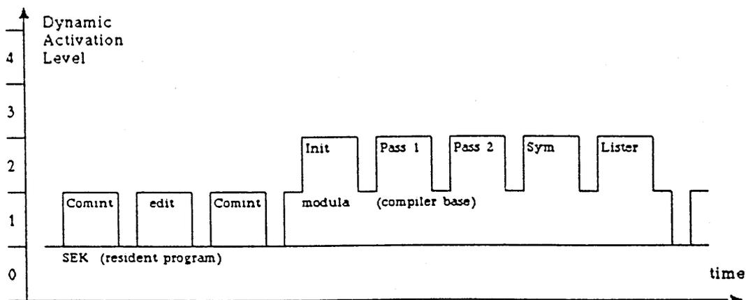
The figure illustrates, how programs may be activated. At a certain moment, the *dynamic activation level* or simply the *level* identifies an active program in the stack.
