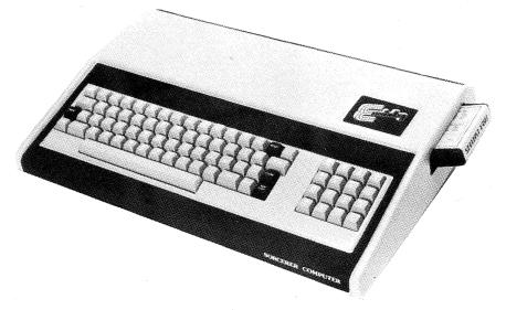
**CAUTION:** Cartridges should be inserted or removed from Sorcerer ONLY when the AC power is off, to protect the programs.
