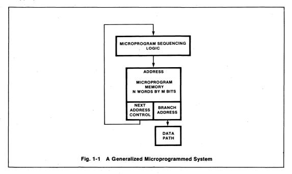
The microprogram memory is simply an N-word by M-bit memory used to hold the various microinstructions. Each word of the microprogram memory contains M bits, which are usually grouped into various fields. The field can consist of various numbers of bits. The definition of the various fields of microprogram word is referred to as FORMATTING. *Figure 1-2* illustrates the format of a 32-bit microprogram word containing nine fields.
