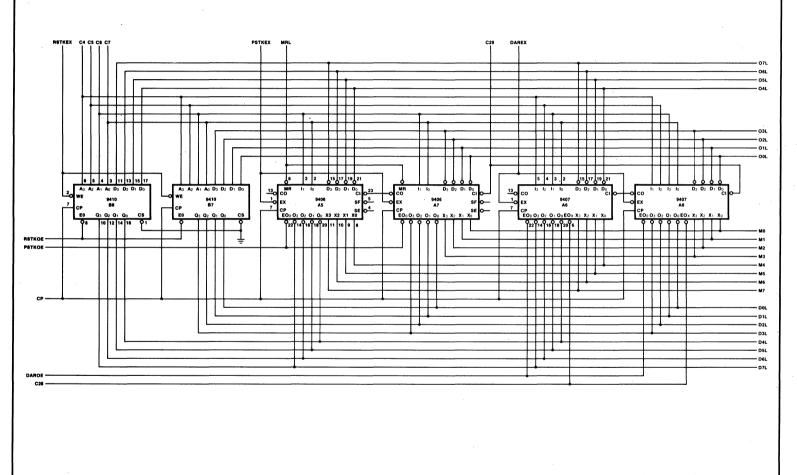
Fig. 3-14 Data Path II Schematic
