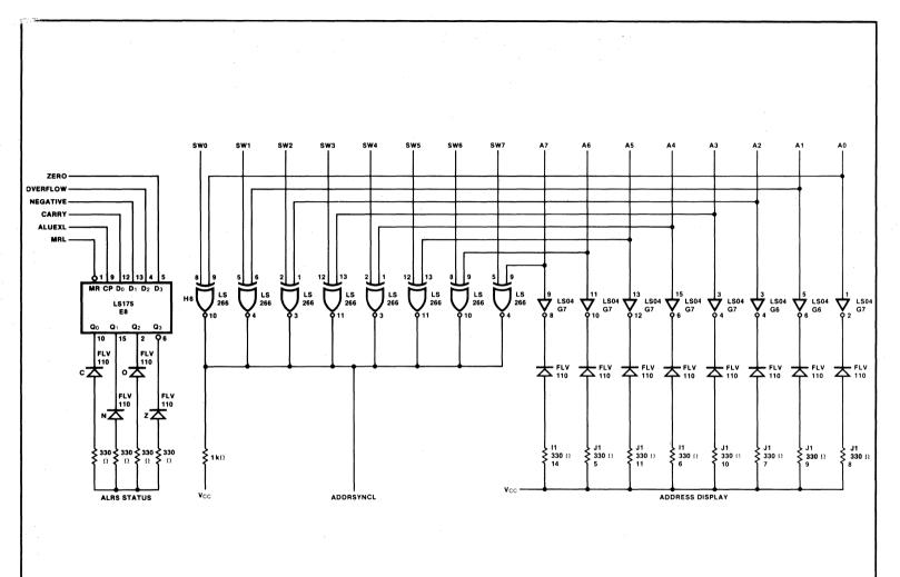
Fig. 3-11 Address Sync, ALRs Flags and Address Display Schematic
