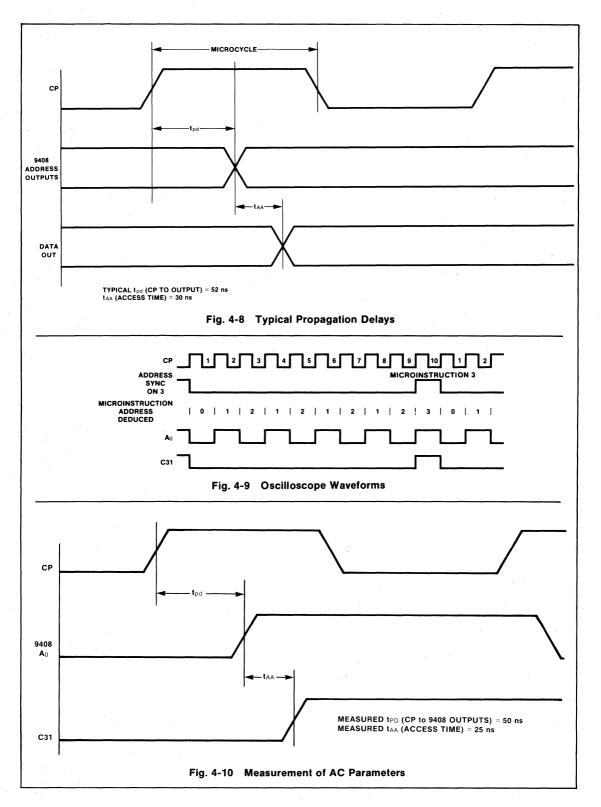
measured as the interval between the rising edge of  $A_0$  and the LOW to HIGH transition of C31. The measured values of the clock to output delay of the 9408 and the address access time of the microprogram memory are 50 and 25 ns, respectively.
