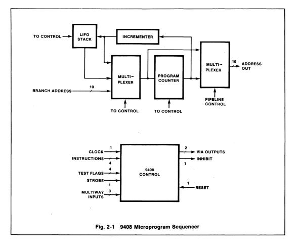
The third type is the *multiway branch*. The multiway branch is similar to an unconditional branch in that a program counter will always be loaded into a specified address, i.e., a branch is certain to occur. However, the address of the branch is determined by substituting the three least significant bits of the branch address present at the input bus by the value of three multiway (test) inputs. The result is that the branch will be made to one of eight different locations.
