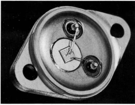
*Power Transistor Package with Chip*
