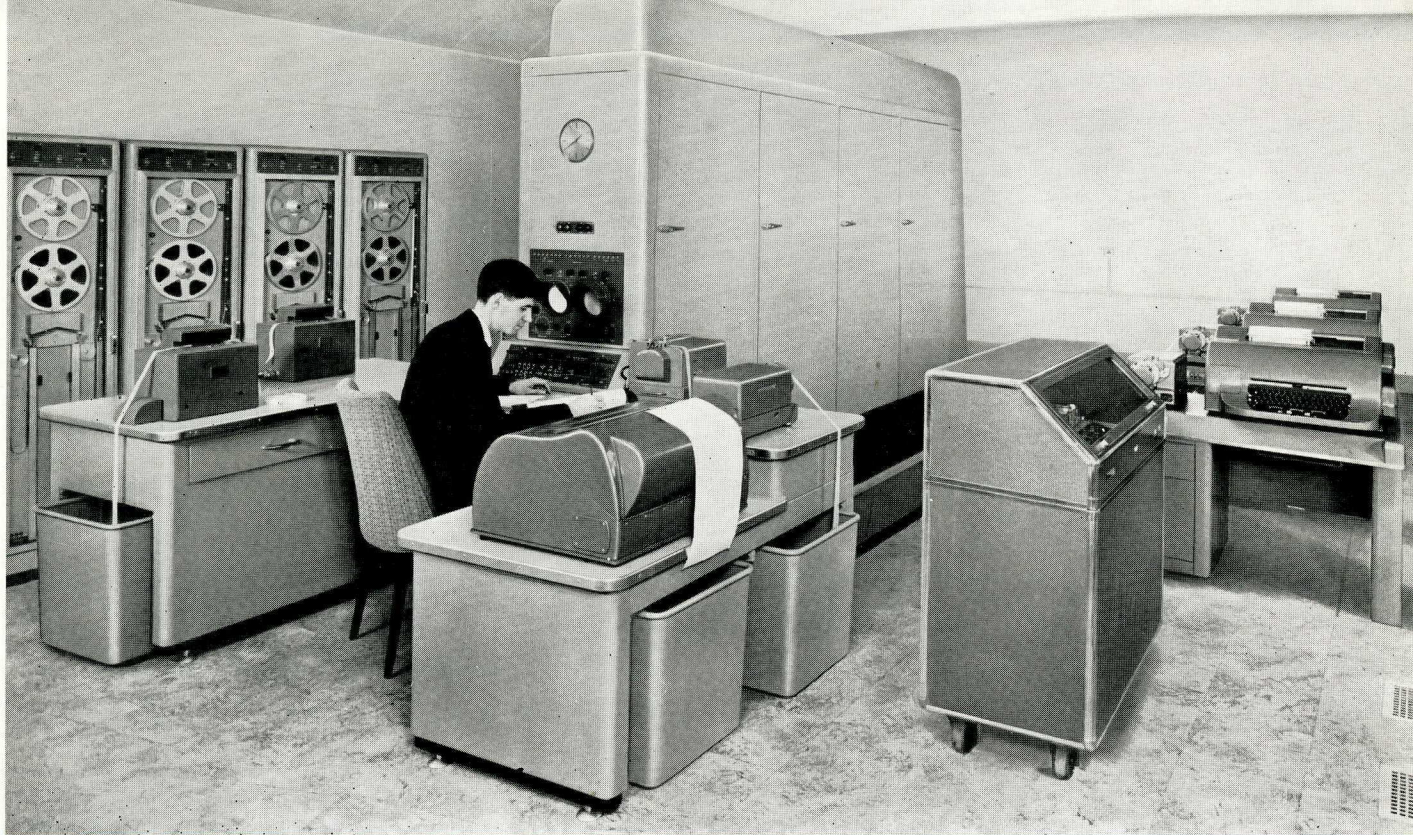
The TR5 is used in the Pegasus Common-Language Data-Processing System which employs high speed paper tape input and output.
