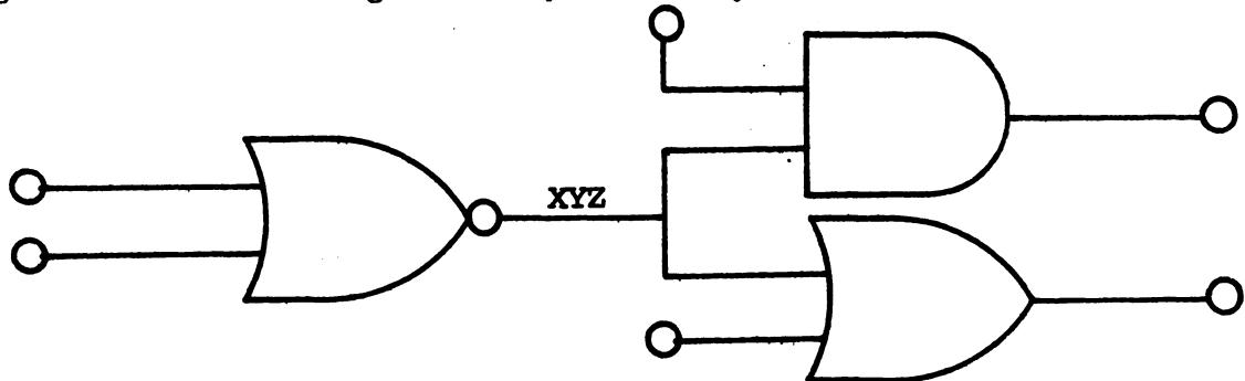
Here XYZ identifies the interconnection between the NOR gate and the AND and OR gates.
