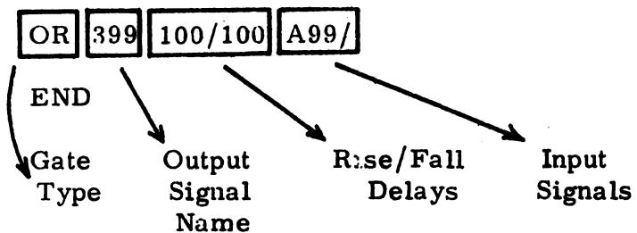
One gate description is entered on each line. Each entry is separated by one or more bl ks. There must be no blanks within the rise/fall entry.
