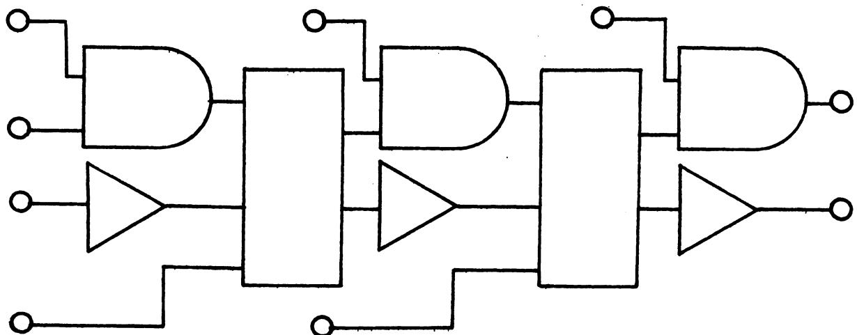
Logic simulation is the process of analyzing the performance of either modules or systems to ensure that they will work correctly once fabricated. These analyses not only evaluate the logical correctness of the design but also the effect of delays in each of the gates or modules.
