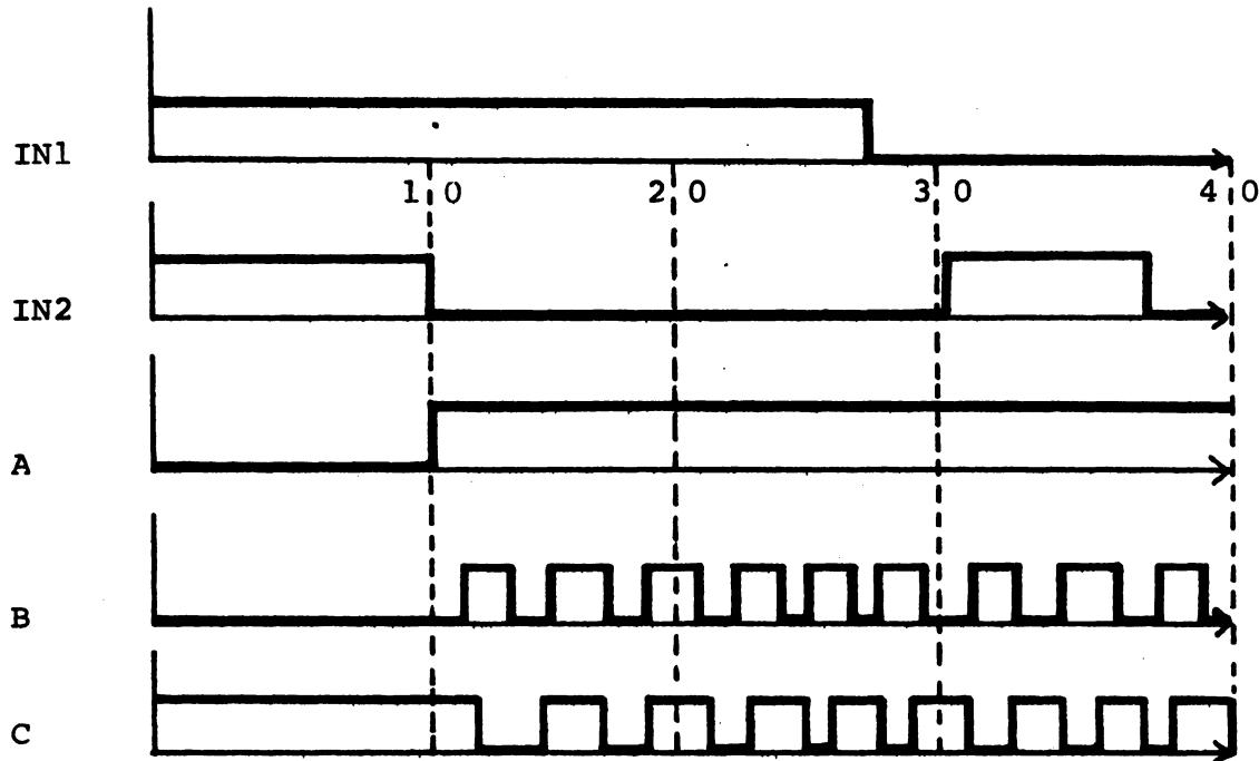
This is achieved by using a time wheel simulation technique. In this, events are placed on a time wheel every time a signal changes state.
