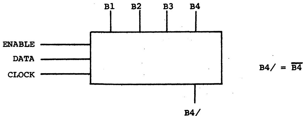
Serial load, parallel or serial out.
