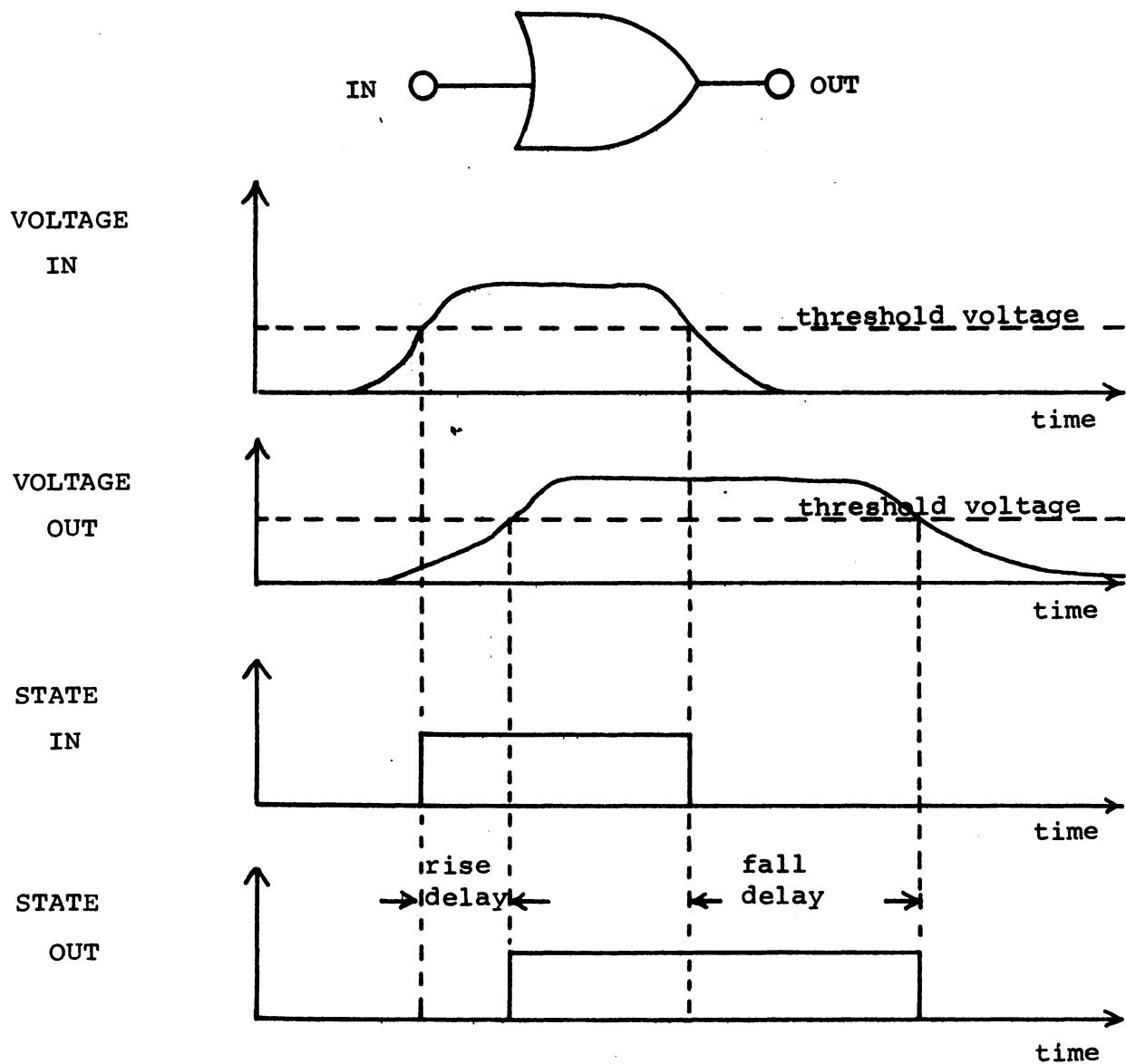
Because the simulator has only two states, the times are taken as those of which the circuit voltages cross the threshold from one state to the other. This threshold is the voltage at which the gates or modules switch states, and the rise and fall delays are specified as shown on the preceding diagram.
