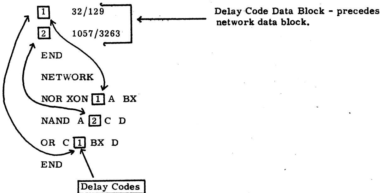
This can save typing if the same rise/fall delay is used many places in the network. Also when the user wishes to change that delay, only the delay code line need be changed.
